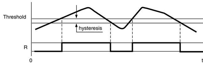
The voltage threshold SR Relay controls a voltage supply which is its own supply. The output relay is energized when the supply (effective for AC) exceeds the selected threshold. It de-energizes when the controlled supply falls below (5 to 20% Hysteresis) of the supply voltage or when the input power breaks. Hysteresis is controlled by a potentiometer and its selection does not change the chosen threshold. Pulses or drops of 100ms or less are ignored.
