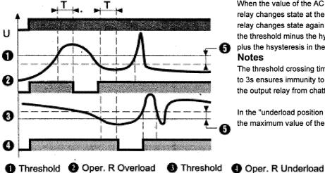
When the value of the AC / DC current reaches the set threshold value the output relay changes state at the end of the time delay T1 (contacts 11 & 14 open). The relay changes state again (contacts 11 & 14 closed) when the current falls below the threshold minus the hysteresis in the overload position, or above the threshold plus the hsysteresis in the underload position.
