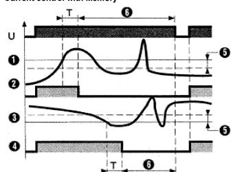
When the value of the AC / DC current reaches the set threshold value the output relay changes state at the end of the time delay T1 (contacts 11 & 14 open) and remains in that condition.
