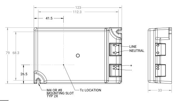
Dimensions for all the LMD125 diagrams are in mm and are for reference only. For exact dimensions and tolerances, refer to the 3-D models (.STEP files) for the LMD125 drivers available by selecting the Documentation tab on the LMH2 product page.
