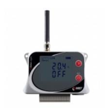
GSM Datalogger is designed to record from two external temperature probes and two two-state inputs. In case of exceeded set limits, SMS and JSON messages can be sent via GPRS data connection. Measured values can be sent to the internet storage <a href="COMET Cloud">COMET Cloud</a>, which is a complete monitoring, alarm and analysis system.
