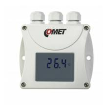
Temperature transmitter for Pt1000/3850ppm sensor is built in a durable watertight case. Degrees Celsius and Fahrenheit are user selectable. Large dual line LCD is an advantage. Display is possible to switch off. Computerized design ensures maximum long term stability and failure indication.
