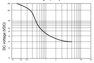
Switching Current (A) resistive load
