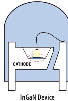
Note: Electrical connection between bottom surface of LED die and the lead frame is achieved through conductive paste.
