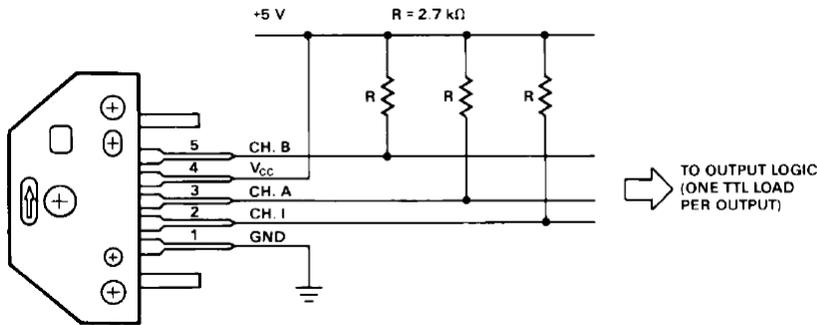
Figure 1. Pull-up Resistors on HEDS-9X40 Encoder Module Outputs.
