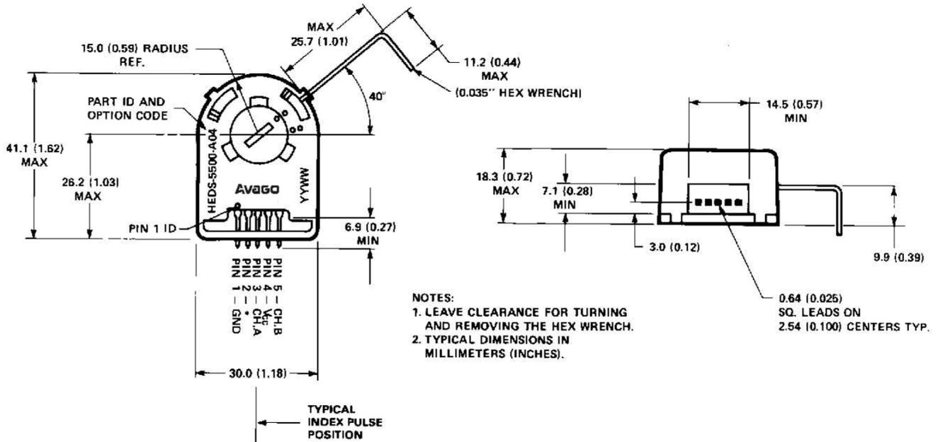
\*Note: For the HEDS-5500 and HEDM-5500, Pin #2 is a No Connect. For the HEDS-5540 and HEDM-5540, Pin #2 is CH. I, the index output.
