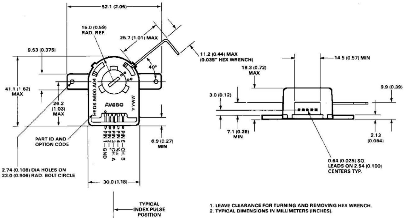
\*Note: For the HEDS-5600 and HEDM-5600, Pin #2 is a No Connect. For the HEDS-5640, Pin #2 is CH. I, the index output.
