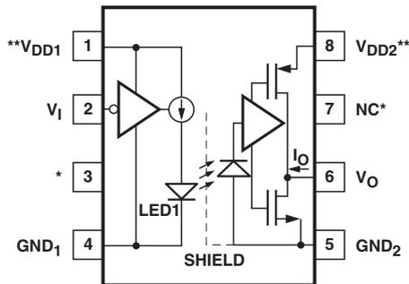
\* Pin 3 is the anode of the internal LED and must be left unconnected for guaranteed data sheet performance. Pin 7 is not connected internally.
