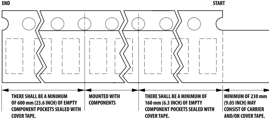
THERE SHALL BE A MINIMUM OF 600 mm (23.6 INCH) OF EMPTY COMPONENT POCKETS SEALED WITH COVER TAPE.
