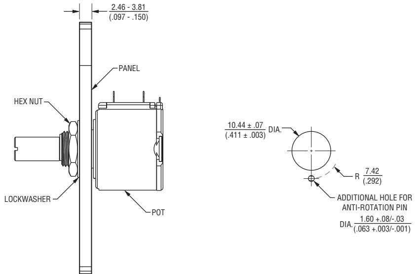
Anti-rotation pin hole is shown at six o'clock position for reference only. The actual location is determined by the customer's application. Refer to the front view of the potentiometer to see the location of the optional A/R pin.
