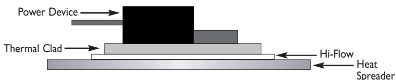
High Power Application Hi-Flow with Thermal Clad
