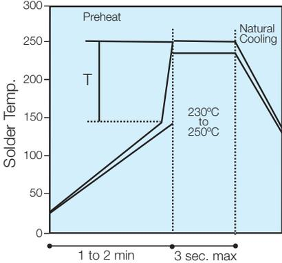
(Preheat chips before soldering)
