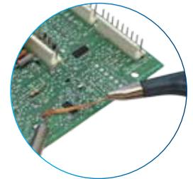
Quickly removes excess solder
