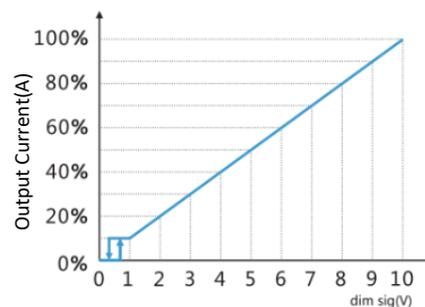
Note: Without 0-10V dimming signal, will run in full power, 0-10V short circuit cut off. The dimmer <0.5mA @10V. Input and output cable may vary as per actual selling area. Contact Autec Sales for any questions
