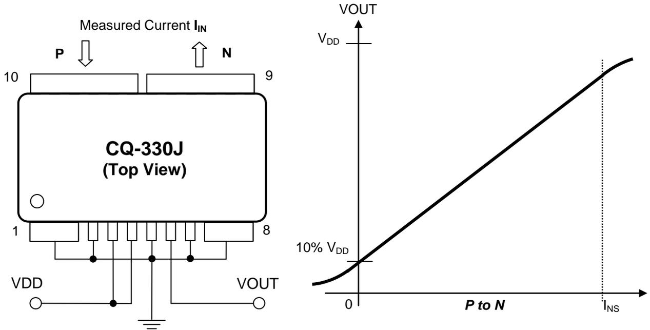
**Figure 2. Pin assignment and typical output characteristics of CQ-330J**
