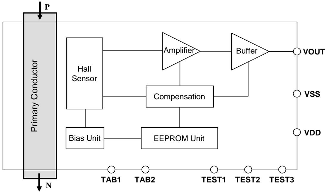
**Figure 1. Functional block diagram of CQ-330J**
