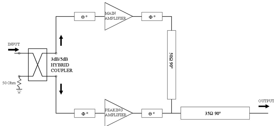
Hybrid coupler can be used in Doherty power amplifier to split the input power into the desired power ratio and phase delay. In above symmetrical Doherty power amplifier (main and peaking amplifier delivers equal amount output power at max drive condition), 3dB hybrid splits the input power into 1:1 ratio with 90 degree phase difference.
