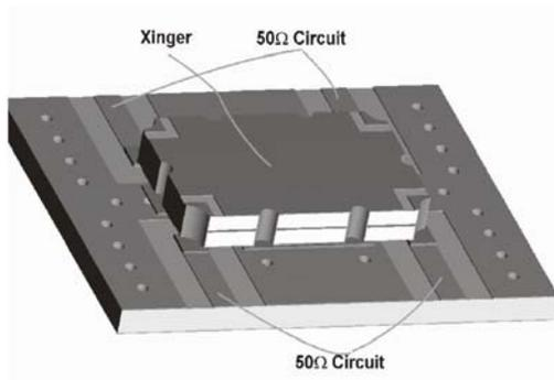
**Figure 3: Component Placement**
