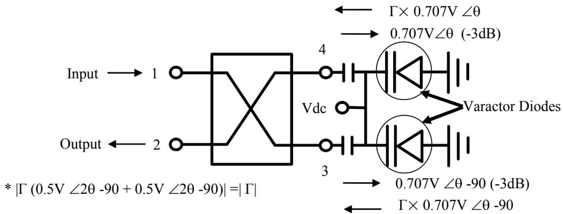
\* The phase angle of the signal exiting port 2 will vary with the phase angle of  $\Gamma$ , which is the reflection angle from the varactor. The varactors must be matched so that their reflection coefficients are equal.
