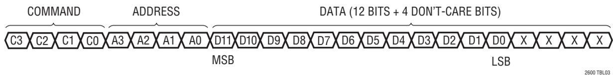
32-bit sequence. The 32-bit word is required for daisy-chain operation, and is also available to accommodate microprocessors which have a minimum word width of 16 bits (2 bytes).
