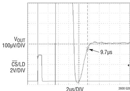
$V_{CC} = 5V$ ,  $V_{REF} = 4.096V$
