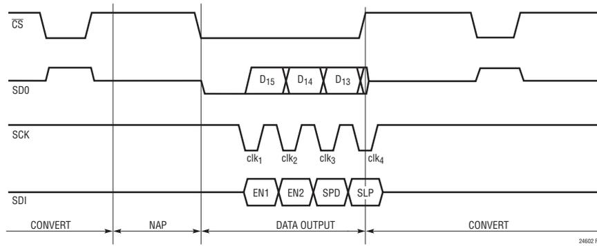
Figure 10. Idle-High (CPOL = 1) Clock and Aborted I/O Example
