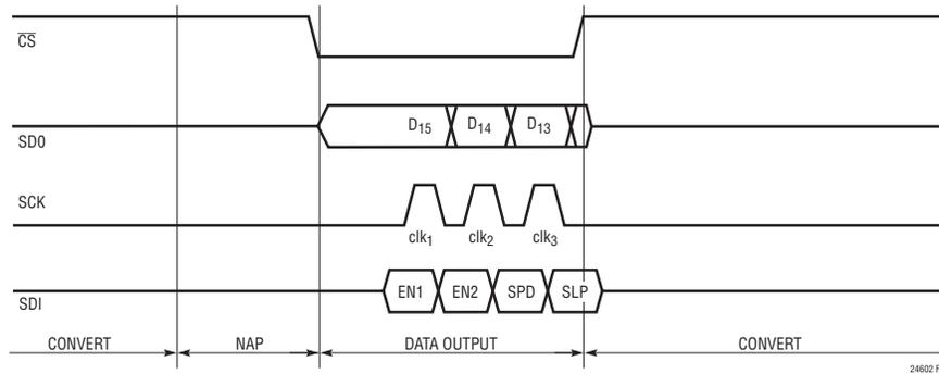
Figure 11. Idle-Low (CPOL = 0) Clock and Aborted I/O Example
