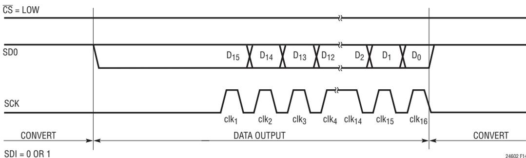
Figure 14. 2-Wire, Idle-Low (CPOL = 0) Serial Clock Operation Example
