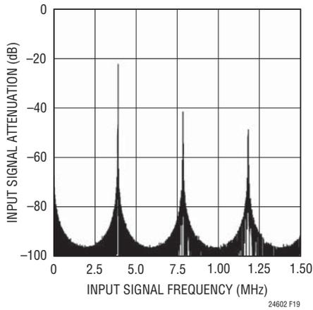
Figure 19. LTC2462 Input Signal Attenuation vs Frequency
