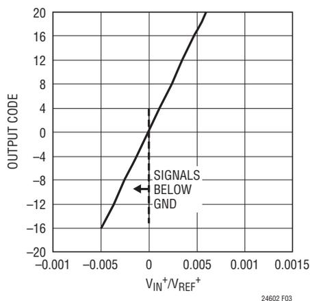
Figure 3. Output Code vs  $V_{\text{IN}^+}$  with  $V_{\text{IN}^-} = 0$  (LTC2462)
