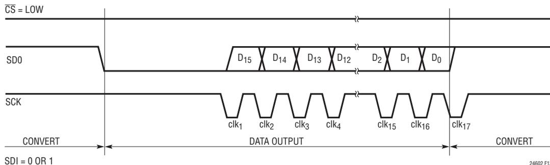
Figure 13. 2-Wire, Idle-High (CPOL = 1) Serial Clock, Operation Example
