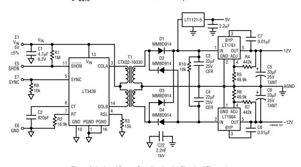
Figure 3. Isolated Power Supplies for the Circuit of Figure 4
