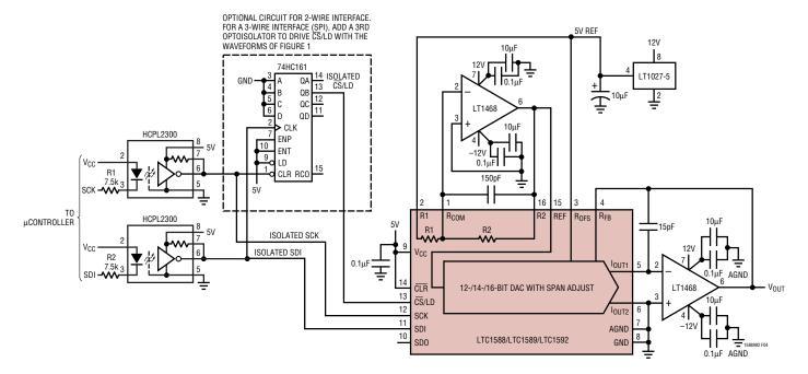
Figure 4. Optically Isolated 16-Bit SoftSpan System
