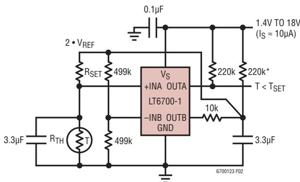
$R_{TH} = 1M$  (e.g., YSI 44015,  $1.00M\Omega$  AT  $25^\circ C$ )
