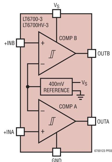
**OUTA:** Open-Collector Output of Comparator Section A. This pin provides drive for up to 40mA of load current. Off-state voltage may be as high as 18V (36V for LT6700HV) above GND, regardless of  $V_S$  used.
