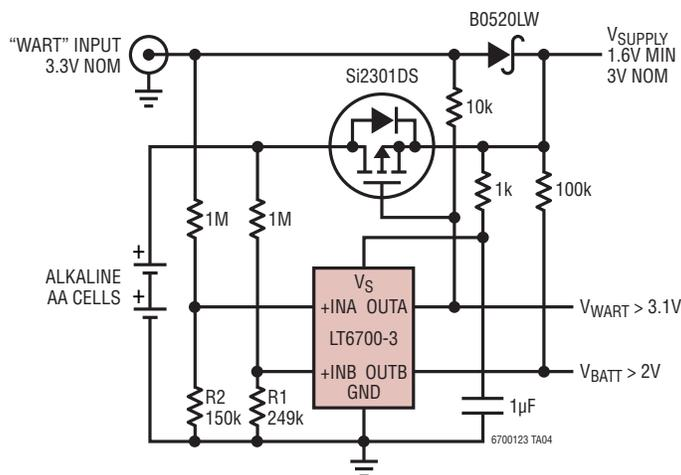
$R1 = 400k / (V_{BATT \text{ AT LOW}} - 0.4)$
