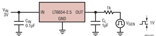
Figure 3. Load Current Response Time Test Circuit
