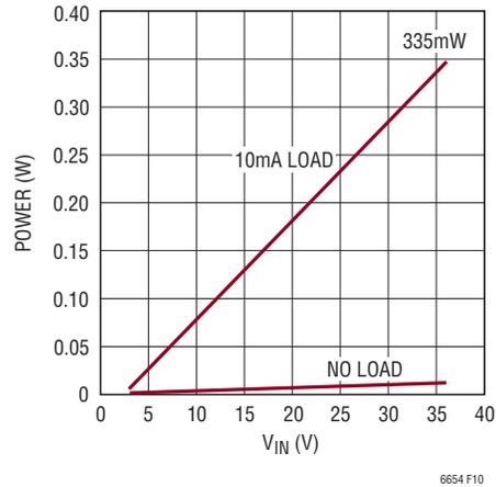
Figure 10. Typical Power Dissipation of the LT6654
