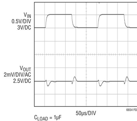
Figure 2. Output Response to 0.5V Ripple on  $V_{\text{IN}}$
