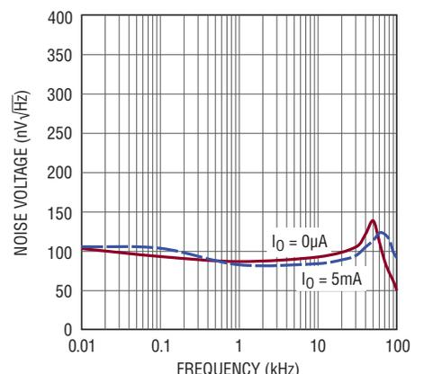
**TYPICAL PERFORMANCE CHARACTERISTICS** The characteristic curves are similar across the LT6654 family. Curves from the LT6654-1.25, LT6654-2.5 and the LT6654-5 represent the full range of typical performance of all voltage options. Characteristic curves for other output voltages fall between these curves and can be estimated based on their output.
