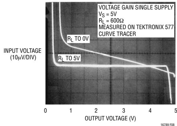
Figure 8. Voltage Gain Single Supply
