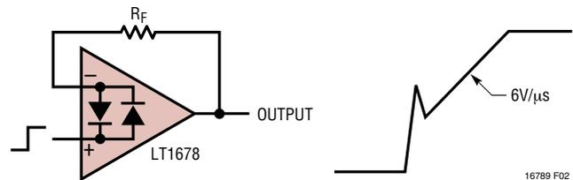
Figure 2. Pulsed Operation
