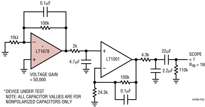
Figure 3. 0.1Hz to 10Hz Noise Test Circuit
