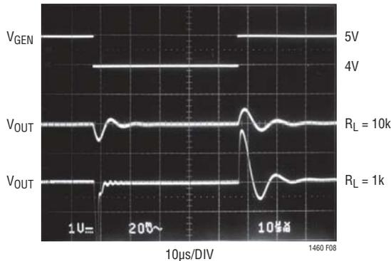
Figure 8.  $C_L = 0.01\mu\text{F}$
