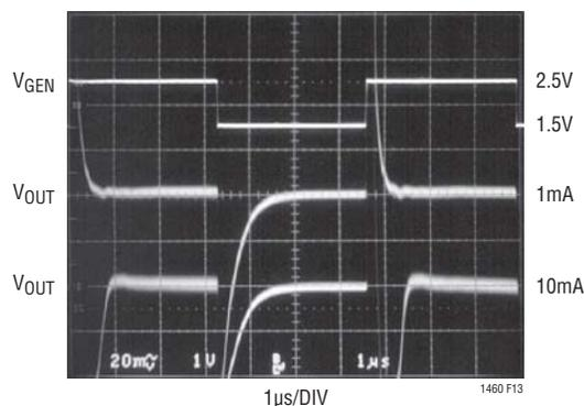
Figure 13.  $C_L = 0\mu$ F
