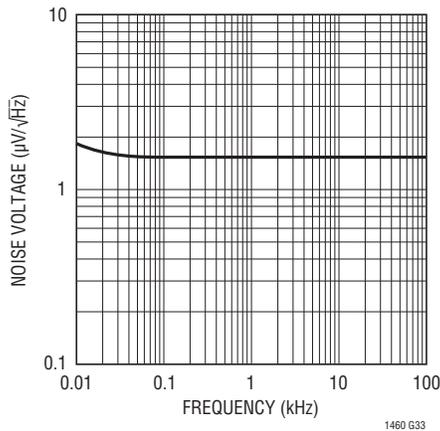
**10V Output Noise 0.1Hz to 10Hz**
