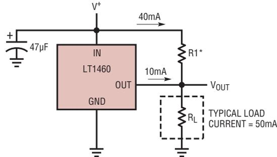
\*SELECT R1 TO DELIVER 80% OF TYPICAL LOAD CURRENT. LT1460 WILL THEN SOURCE AS NECESSARY TO MAINTAIN PROPER OUTPUT. DO NOT REMOVE LOAD AS OUTPUT WILL BE DRIVEN UNREGULATED HIGH. LINE REGULATION IS DEGRADED IN THIS APPLICATION
