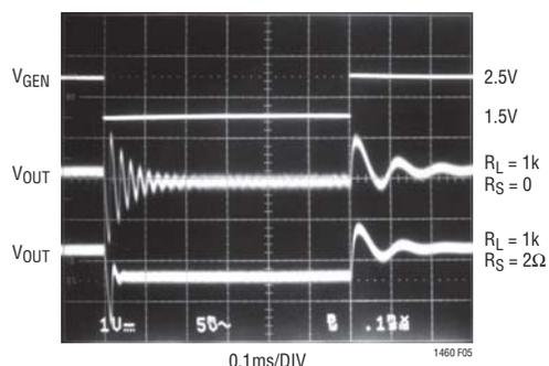
Figure 5. Effect of  $R_S$  for  $C_L = 1\mu F$
