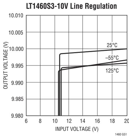
**TYPICAL PERFORMANCE CHARACTERISTICS** Characteristic curves are similar for all voltage options of the LT1460S3. Curves from the LT1460S3-2.5 and the LT1460S3-10 represent the extremes of the voltage options. Characteristic curves for other output voltages fall between these curves, and can be estimated based on their voltage output.
