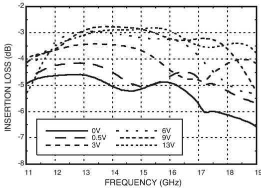
**Insertion Loss vs. Vctl , F = 15 GHz**
