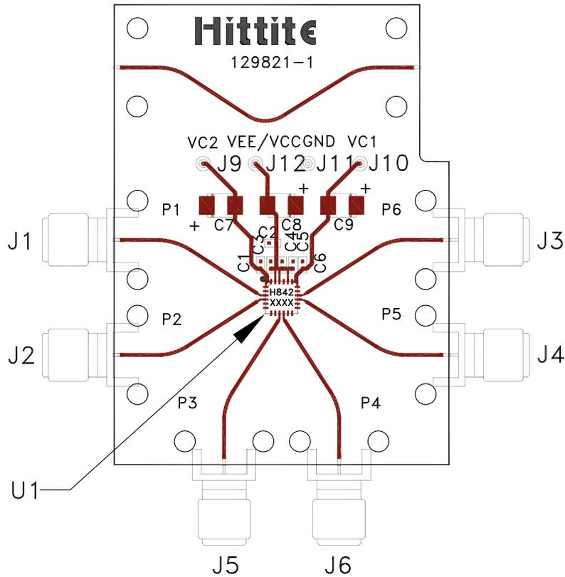
Note: VC1 on evaluation board is VAC2 and VC2 on evaluation board is VAC1
