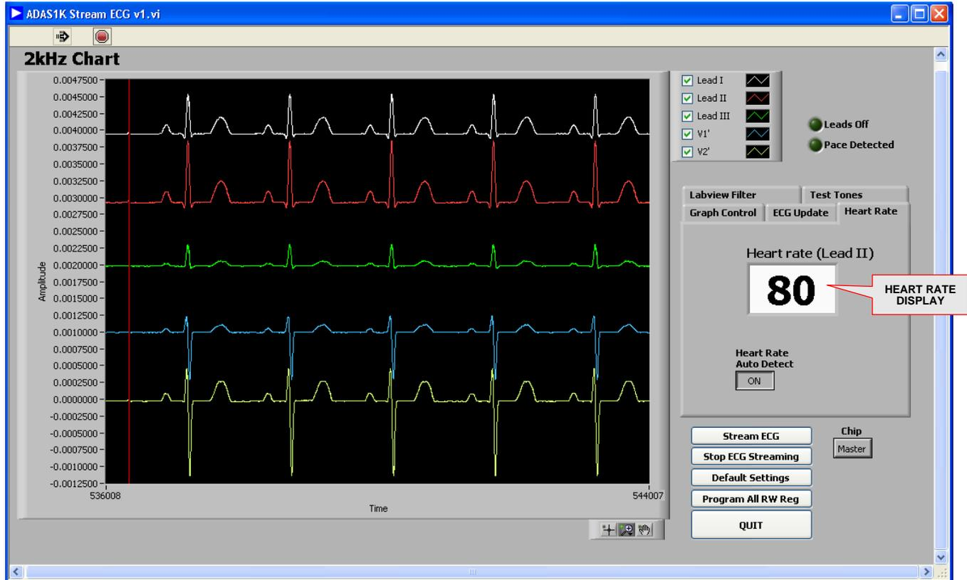
Figure 18. ECG Capture Window with Heart Rate Shown
