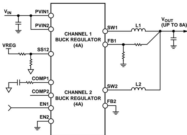
Figure 45. Parallel Operation for Channel 1 and Channel 2
