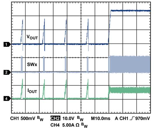
Figure 33. Short-Circuit Protection Recovery,  $V_{IN} = 12\text{ V}$ ,  $V_{OUT} = 1.2\text{ V}$ ,  $f_{SW} = 600\text{ kHz}$ ,  $L = 1\text{ }\mu\text{H}$ ,  $C_{OUT} = 47\text{ }\mu\text{F} \times 2$
