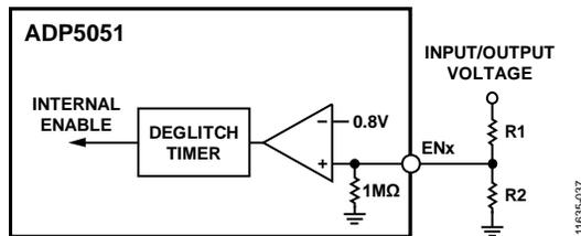
Figure 38. Precision Enable Diagram for a Single Channel
