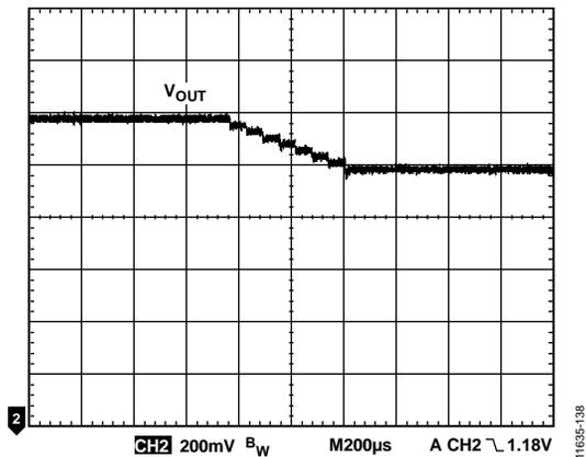
Figure 35. Channel 1 Dynamic Voltage Scaling (DVS) from 1.3 V to 1.1 V, 62.5  $\mu$ s Interval,  $V_{IN} = 12$  V,  $I_{OUT} = 4$  A,  $f_{SW} = 600$  kHz,  $L = 1$   $\mu$ H,  $C_{OUT} = 47$   $\mu$ F  $\times 2$
