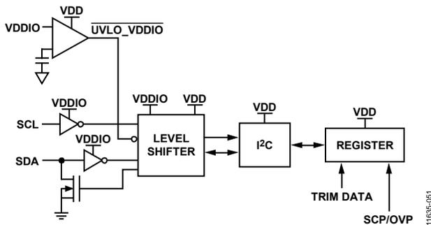
Figure 55. I<sup>2</sup>C Interface Block Diagram
