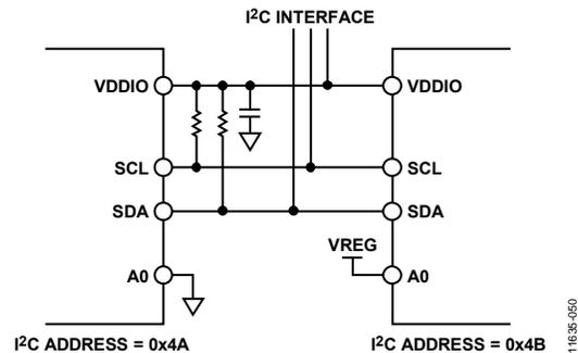
Figure 56. Two **ADP5051** Devices Configured with Different I<sup>2</sup>C Addresses (A0 Function Replaces PWRGD Function on Pin 20)
