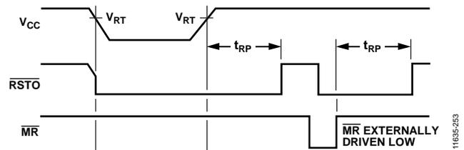
Figure 53.  $\overline{MR}$  Timing Diagram in Processor Reset Mode
