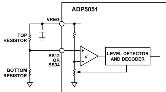
Figure 44. Level Detector Circuit for Soft Start
