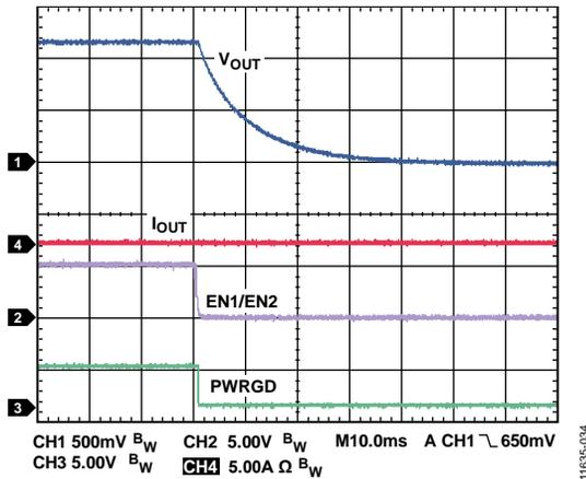
Figure 31. Channel 1/Channel 2 Shutdown with Active Output Discharge,  $V_{IN} = 12\text{ V}$ ,  $V_{OUT} = 1.2\text{ V}$ ,  $f_{SW} = 600\text{ kHz}$ ,  $L = 1\text{ }\mu\text{H}$ ,  $C_{OUT} = 47\text{ }\mu\text{F} \times 2$
