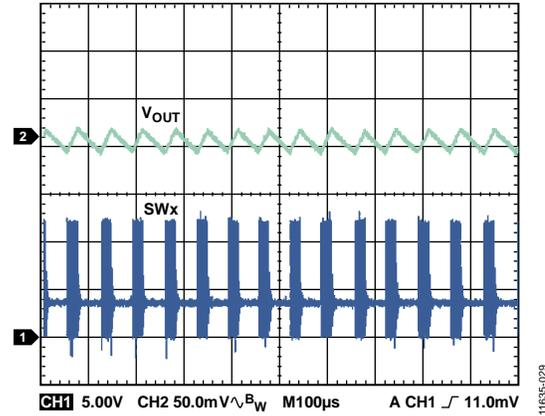
Figure 26. Steady State Waveform at Light Load,  $V_{IN} = 12\text{ V}$ ,  $V_{OUT} = 3.3\text{ V}$ ,  $I_{OUT} = 30\text{ mA}$ ,  $f_{SW} = 600\text{ kHz}$ ,  $L = 4.7\text{ }\mu\text{H}$ ,  $C_{OUT} = 47\text{ }\mu\text{F} \times 2$ , Automatic PWM/PSM Mode
