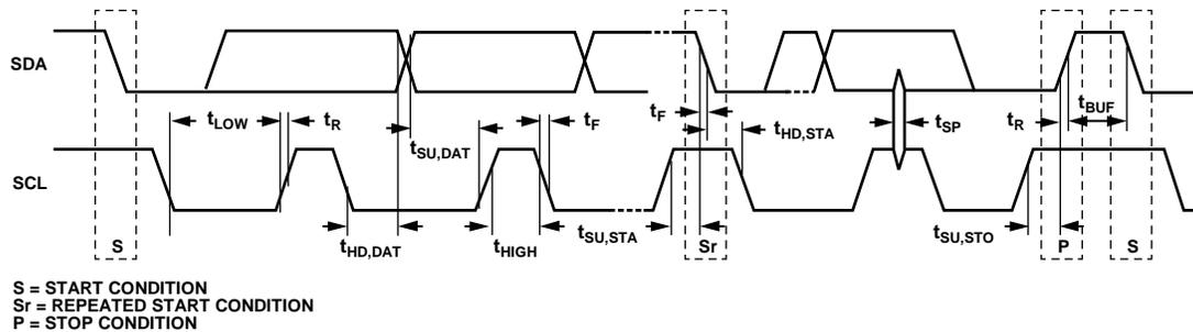
Figure 3. I<sup>2</sup>C Interface Timing Diagram
