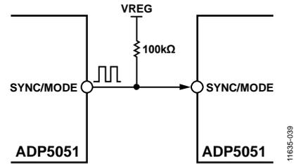
Figure 42. Two ADP5051 Devices Configured for Synchronization Mode
