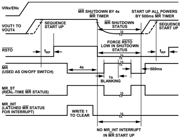
Figure 54.  $\overline{MR}$  Timing Diagram in Power-On/Off Switch Mode
