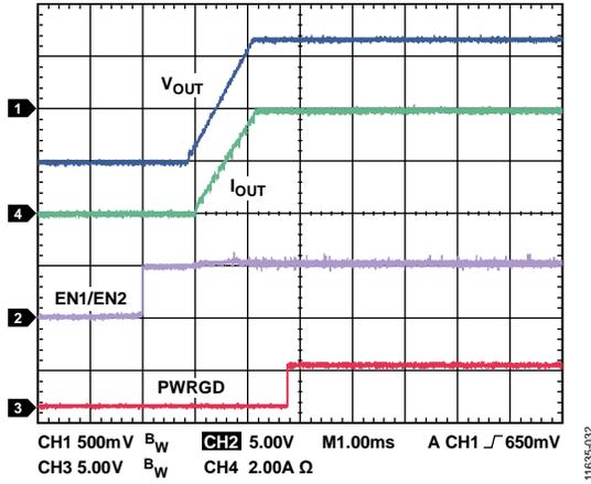
Figure 29. Channel 1/Channel 2 Soft Start with 4 A Resistance Load,  $V_{IN} = 12\text{ V}$ ,  $V_{OUT} = 1.2\text{ V}$ ,  $f_{SW} = 600\text{ kHz}$ ,  $L = 1\text{ }\mu\text{H}$ ,  $C_{OUT} = 47\text{ }\mu\text{F} \times 2$
