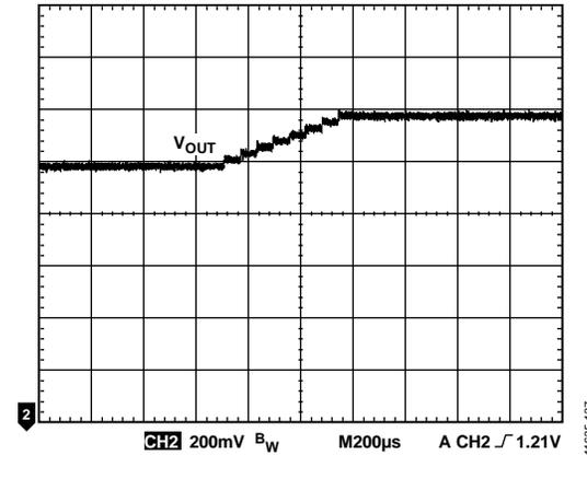
Figure 34. Channel 1 Dynamic Voltage Scaling (DVS) from 1.1 V to 1.3 V, 62.5  $\mu\text{s}$  Interval,  $V_{IN} = 12\text{ V}$ ,  $I_{OUT} = 4\text{ A}$ ,  $f_{SW} = 600\text{ kHz}$ ,  $L = 1\text{ }\mu\text{H}$ ,  $C_{OUT} = 47\text{ }\mu\text{F} \times 2$
