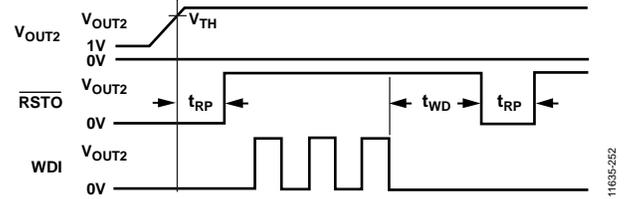
Figure 52. Watchdog Timing Diagram
