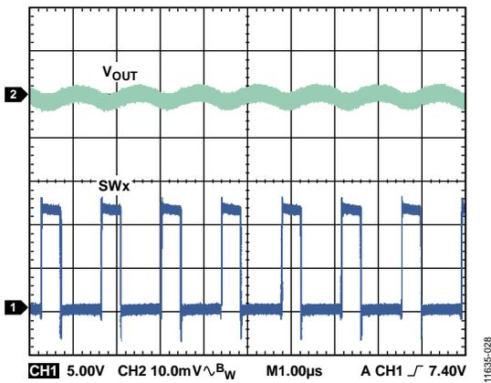
Figure 25. Steady State Waveform at Heavy Load,  $V_{IN} = 12\text{ V}$ ,  $V_{OUT} = 3.3\text{ V}$ ,  $I_{OUT} = 3\text{ A}$ ,  $f_{SW} = 600\text{ kHz}$ ,  $L = 4.7\text{ }\mu\text{H}$ ,  $C_{OUT} = 47\text{ }\mu\text{F} \times 2$ , FPWM Mode
