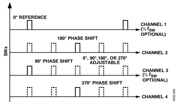
Figure 40. Phase Shift Diagram, Four Buck Regulators
