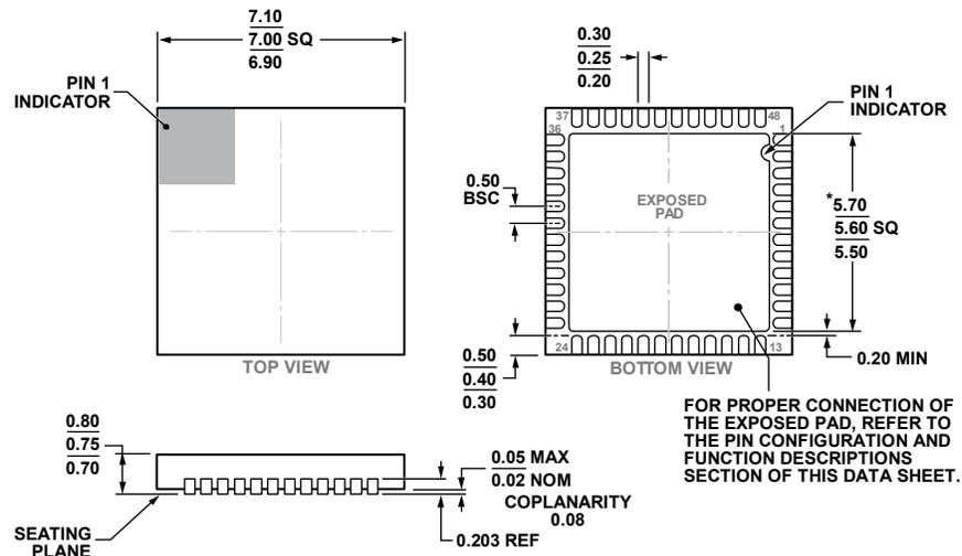
\*COMPLIANT TO JEDEC STANDARDS MO-220-WKGD-2 WITH THE EXCEPTION OF THE EXPOSED PAD DIMENSION.
