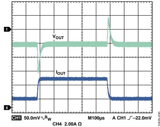
Figure 27. Channel 1/Channel 2 Load Transient, 1 A to 4 A,  $V_{IN} = 12\text{ V}$ ,  $V_{OUT} = 3.3\text{ V}$ ,  $f_{SW} = 600\text{ kHz}$ ,  $L = 2.2\text{ }\mu\text{H}$ ,  $C_{OUT} = 47\text{ }\mu\text{F} \times 2$
