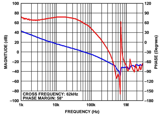
Figure 60. Bode Plot for 1.2 V Output
