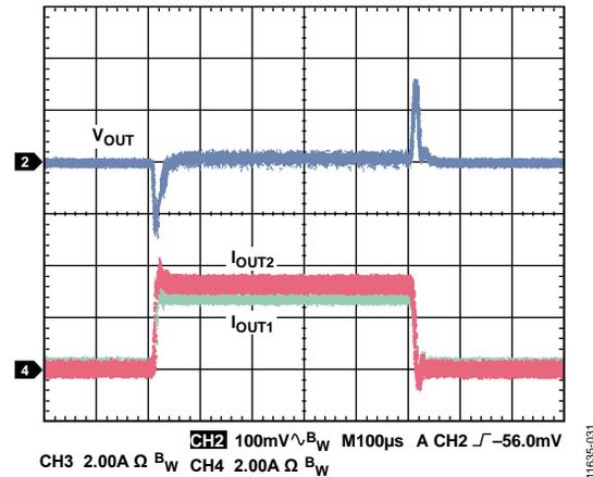
Figure 28. Load Transient, Channel 1/Channel 2 Parallel Output, 0 A to 6 A,  $V_{IN} = 12\text{ V}$ ,  $V_{OUT} = 3.3\text{ V}$ ,  $f_{SW} = 600\text{ kHz}$ ,  $L = 4.7\text{ }\mu\text{H}$ ,  $C_{OUT} = 47\text{ }\mu\text{F} \times 4$
