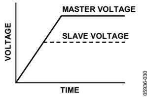
Figure 31. Coincident Tracking
