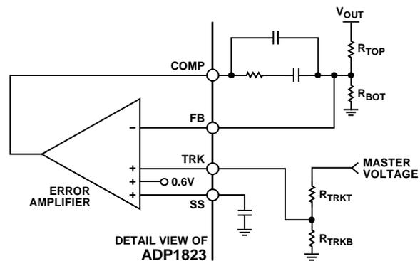
Figure 30. Voltage Tracking
