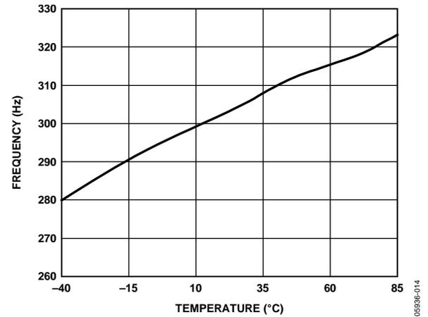
Figure 14. Switching Frequency vs. Temperature,  $V_{IN} = 12\text{ V}$
