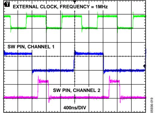
Figure 19. Out-of-Phase Switching, External 1 MHz Clock
