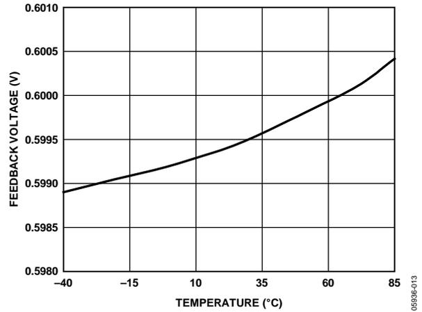
Figure 13. Feedback Voltage vs. Temperature,  $V_{IN} = 12\text{ V}$
