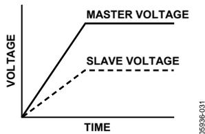
Figure 32. Ratiometric Tracking
