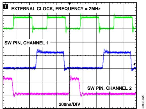
Figure 20. Out-of-Phase Switching, External 2 MHz Clock
