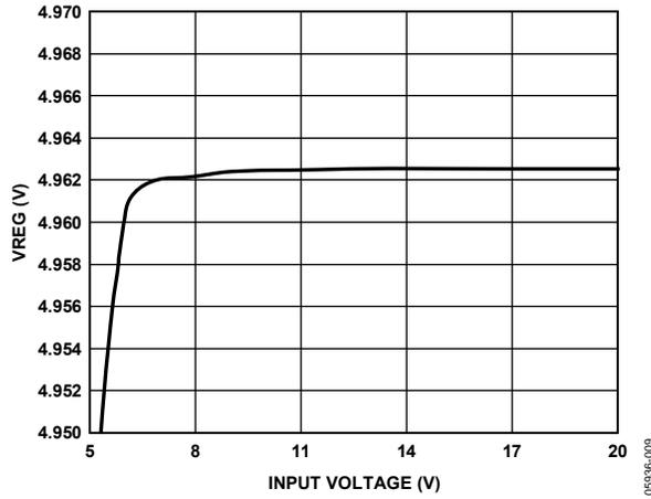
Figure 9. VREG vs. Input Voltage, 10 mA Load
