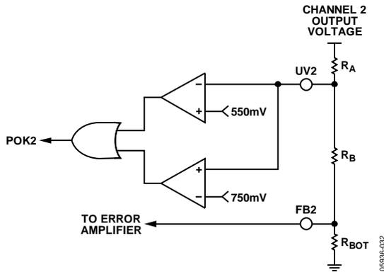
Figure 33. Setting the Channel 2 Undervoltage Threshold
