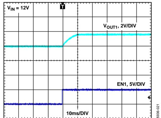
Figure 21. Enable Pin Response,  $V_{IN} = 12 V$
