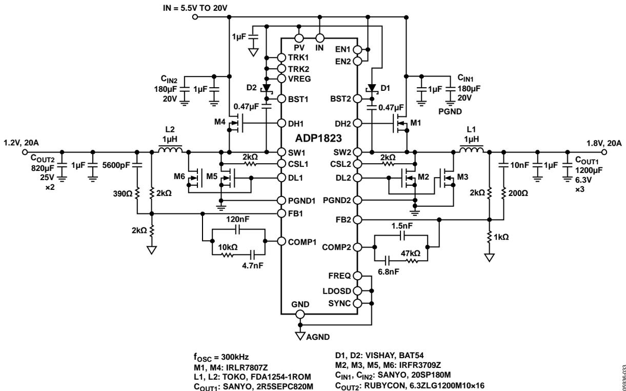
Figure 34. Application Circuit with 20 A Output Loads
