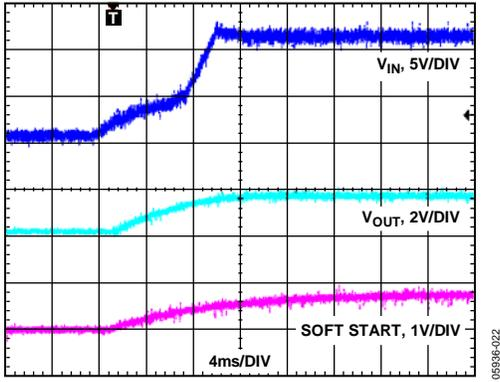
Figure 22. Power-On Response, EN Tied to  $V_{IN}$
