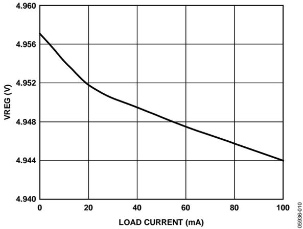
Figure 10. VREG vs. Load Current,  $V_{IN} = 12\text{ V}$
