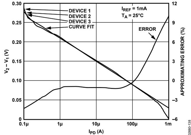
Figure 39.  $V_2 - V_1$  Error vs. Input Current.
