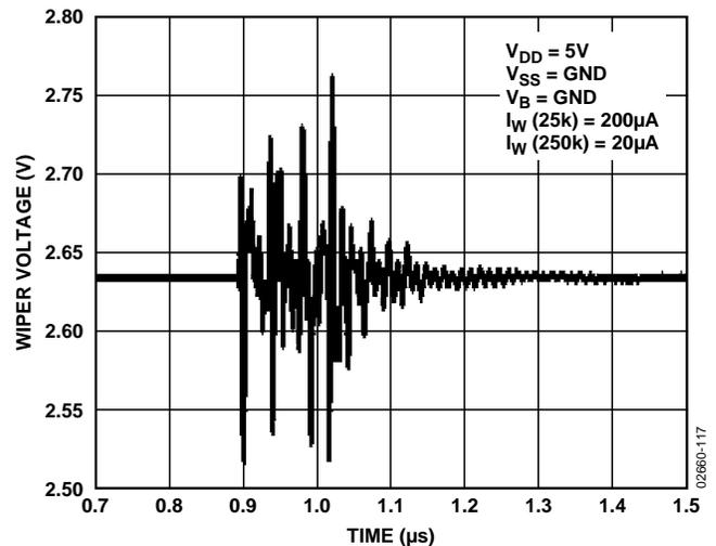
Figure 17. Digital Feedthrough
