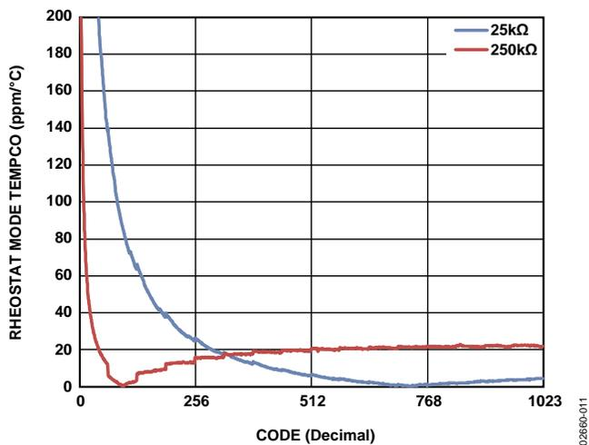
Figure 8.  $(\Delta R_{WB}/R_{WB})/\Delta T \times 10^6$  Rheostat Mode Tempco
