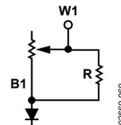
Figure 41. Resistor Scaling with Pseudo Log Adjustment Characteristics
