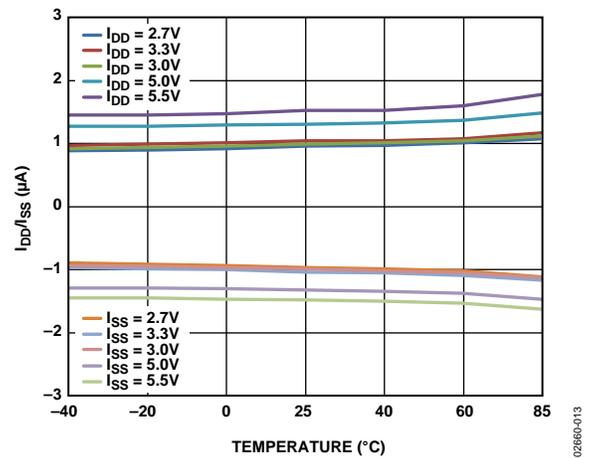
Figure 10.  $I_{DD}$  vs. Temperature,  $R_{AB} = 25\text{ k}\Omega$
