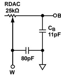
Figure 43. RDAC Circuit Simulation Model (RDAC = 25 kΩ)
