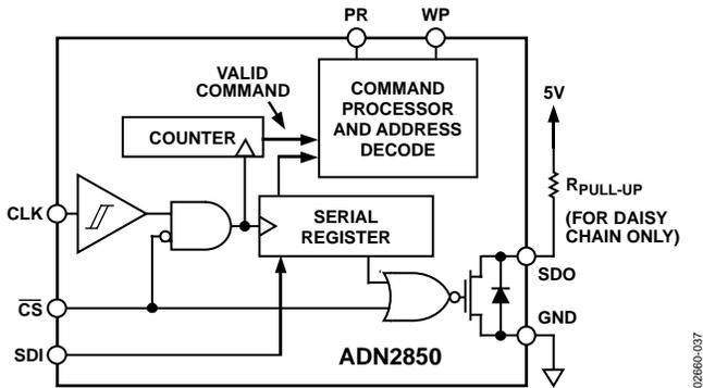
Figure 25. Equivalent Digital Input and Output Logic
