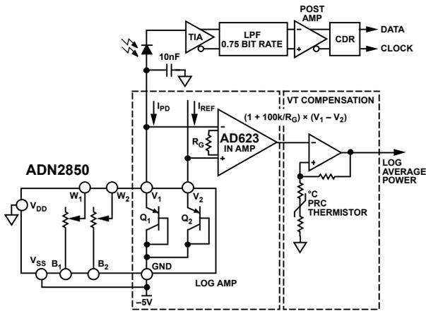
Figure 38. Conceptual Incoming Optical Power Monitoring Circuit
