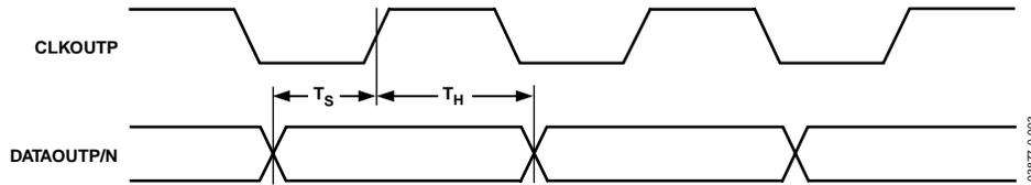
Figure 3. Output Timing
