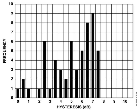
Figure 5. LOS Hysteresis OC-3, -40°C, 3.6 V, 2<sup>23</sup>-1 PRBS Input Pattern, R<sub>TH</sub> = 90 kΩ
