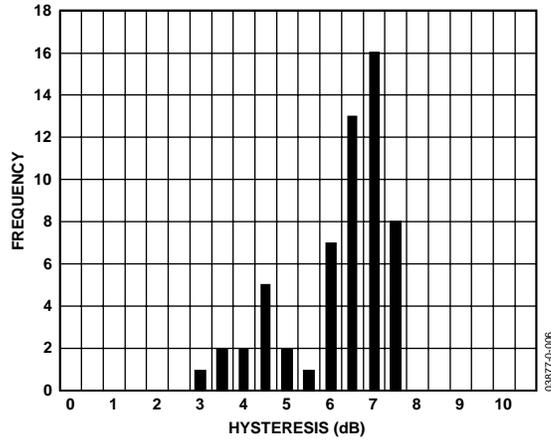
Figure 6. LOS Hysteresis OC-12, -40°C, 3.6 V, 2<sup>23</sup>-1 PRBS Input Pattern, R<sub>TH</sub> = 90 kΩ
