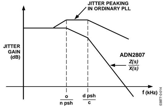
Figure 14. Jitter Response vs. Conventional Phase-Locked Loop
