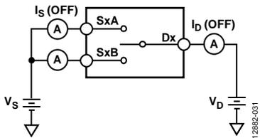
Figure 31. Off Leakage
