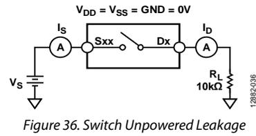
Figure 36. Switch Unpowered Leakage
