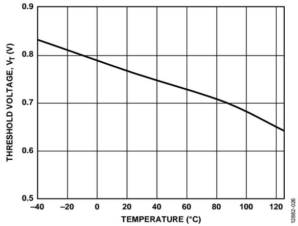
Figure 26. Threshold Voltage ( $V_T$ ) vs. Temperature
