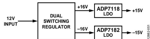
Figure 51. Bipolar Power Solution
