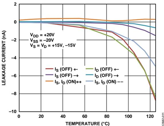
Figure 12. Leakage Current vs. Temperature, ±20 V Dual Supply
