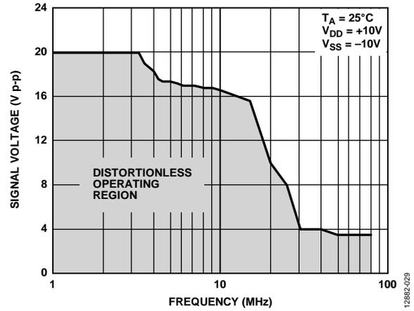
Figure 29. Large Signal Voltage Tracking vs. Frequency
