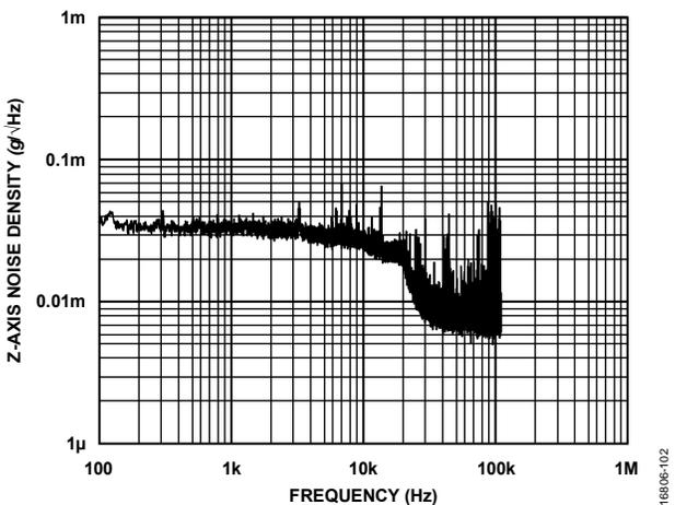
Figure 15. Z-Axis Noise Density, Wideband, RTS Mode
