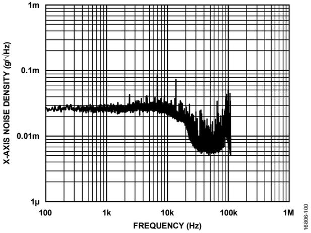
Figure 13. X-Axis Noise Density, Wideband, RTS Mode
