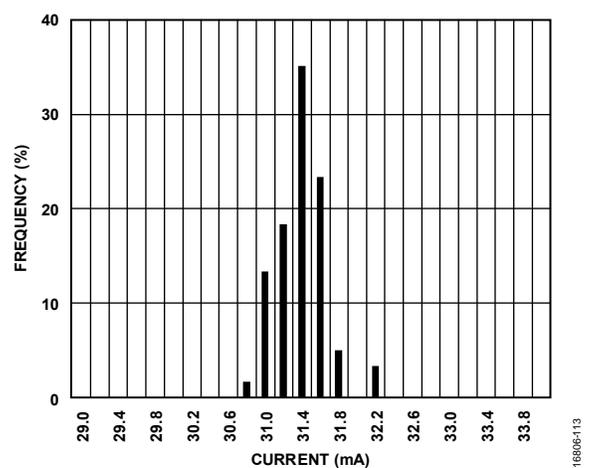
Figure 24. Operating Mode Current Distribution at 3.6 V Supply
