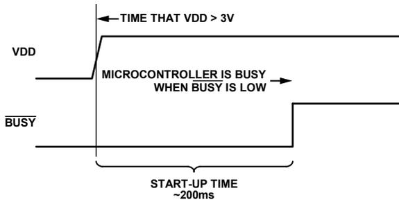
Figure 47.  $\overline{\text{BUSY}}$  Response During Startup
