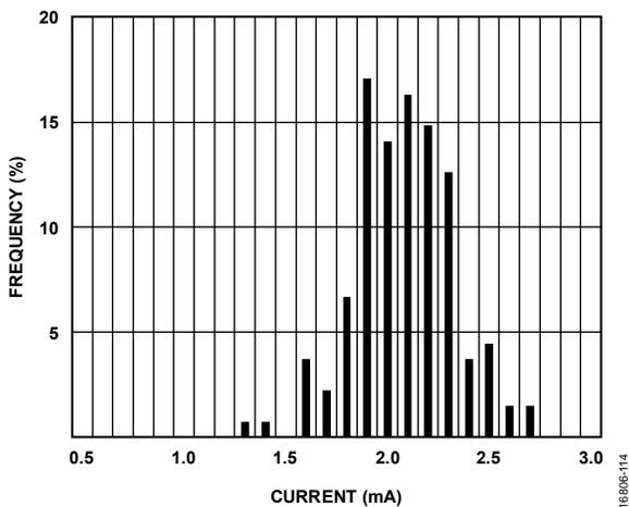
Figure 27. Sleep Mode Current Distribution at 3.6 V Supply
