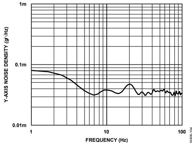
Figure 17. Y-Axis Noise Density, Low Frequency, RTS Mode
