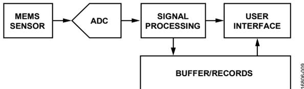
Figure 34. Basic Signal Chain
