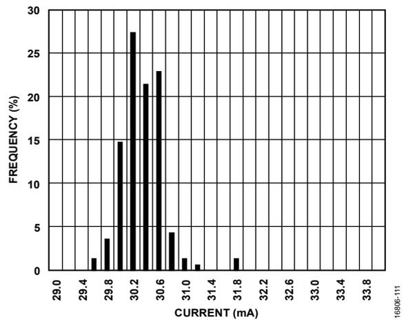
Figure 23. Operating Mode Current Distribution at 3.3 V Supply
