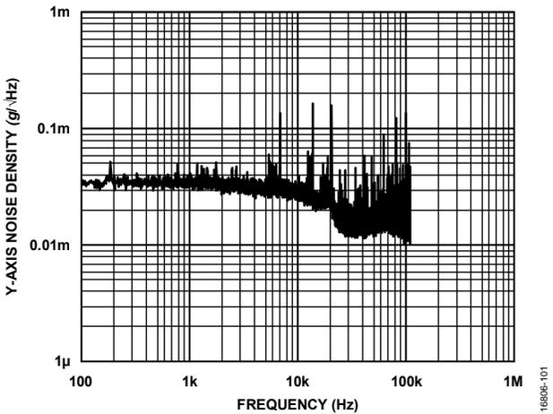
Figure 14. Y-Axis Noise Density, Wideband, RTS Mode
