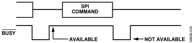
Figure 46. Busy Signal ( $\overline{\text{BUSY}}$ ) Orientation after SPI command
