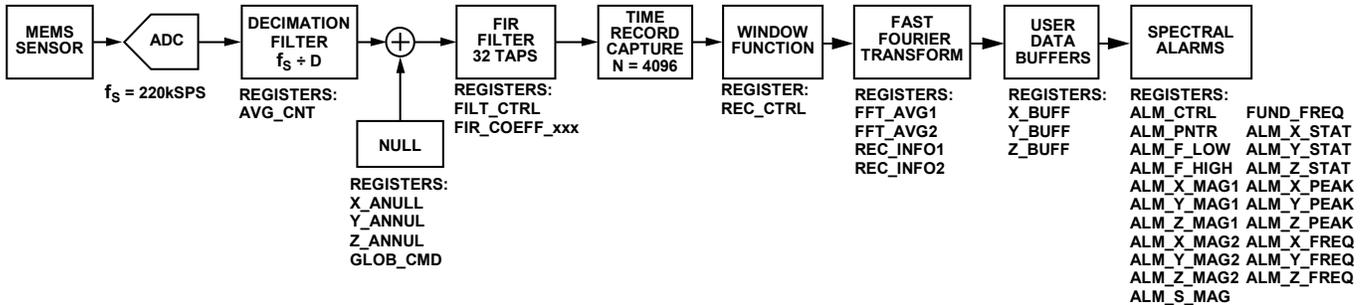
Figure 50. AFFT Mode and MFFT Mode Datapath Processing
