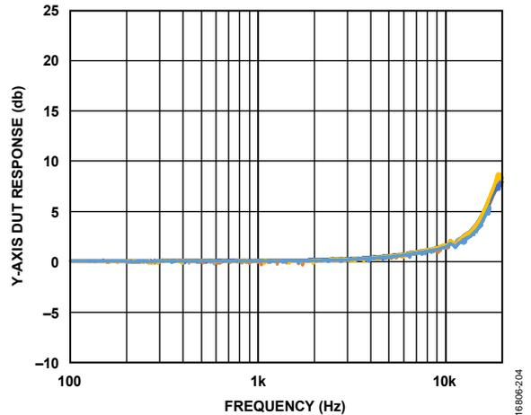
Figure 11. Y-Axis Sine Sweep Response, RTS Mode
