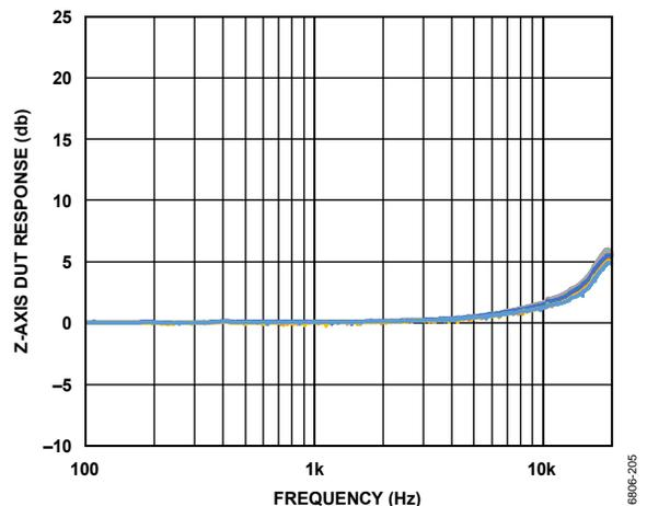
Figure 12. Z-Axis Sine Sweep Response, RTS Mode
