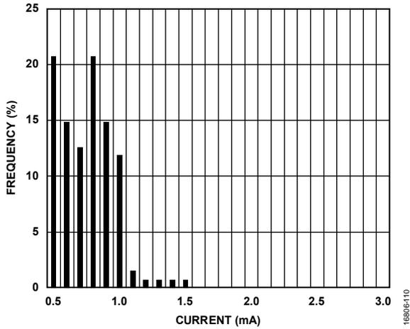
Figure 25. Sleep Mode Current Distribution at 3.0 V Supply
