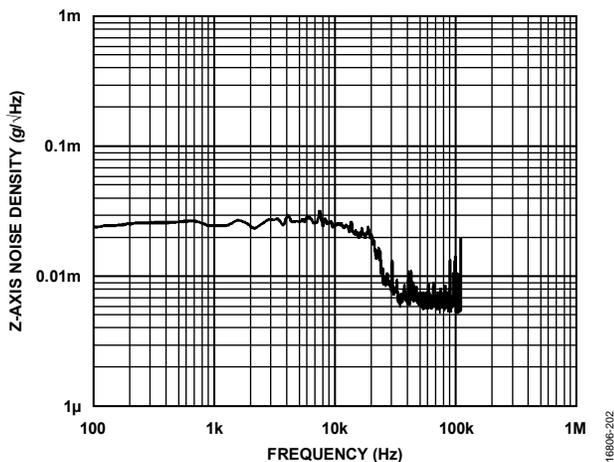
Figure 9. Z-Axis Noise Density, Wideband, MTC, AVG\_CNT = 0
