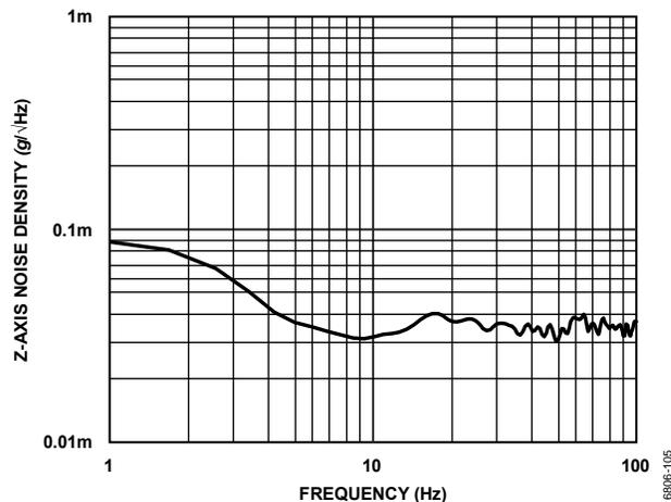
Figure 18. Z-Axis Noise Density, Low Frequency, RTS Mode
