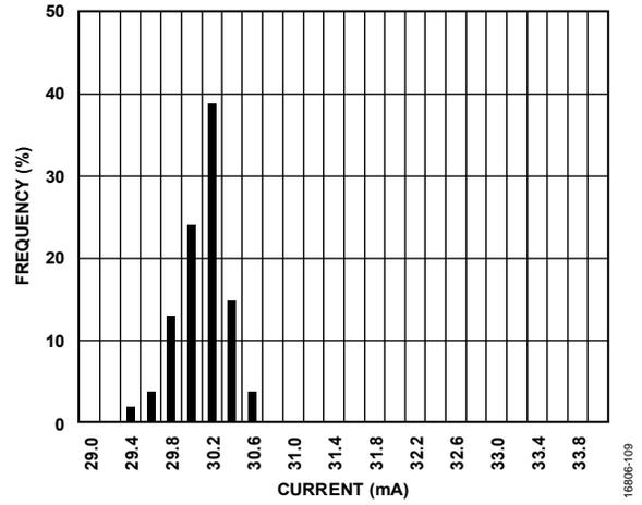
Figure 22. Operating Mode Current Distribution at 3.0 V Supply
