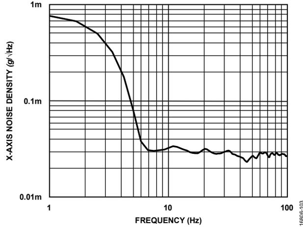
Figure 16. X-Axis Noise Density, Low Frequency, RTS Mode
