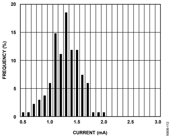
Figure 26. Sleep Mode Current Distribution at 3.3 V Supply
