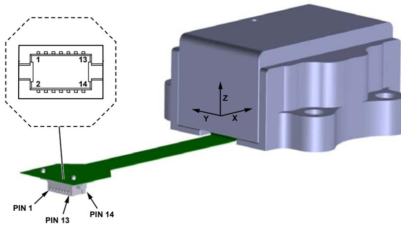
Figure 6. Pin Configuration
