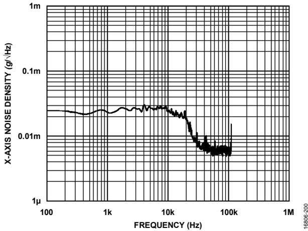
Figure 7. X-Axis Noise Density, Wideband, MTC, AVG\_CNT = 0
