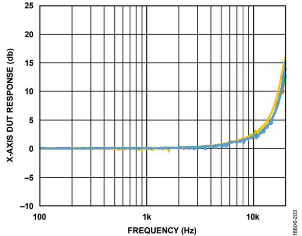
Figure 10. X-Axis Sine Sweep Response, RTS Mode
