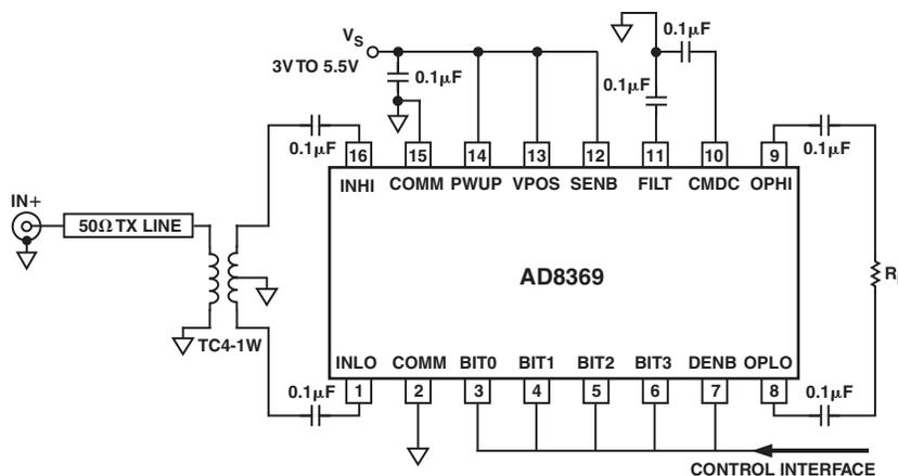
Figure 3. Basic Connections
