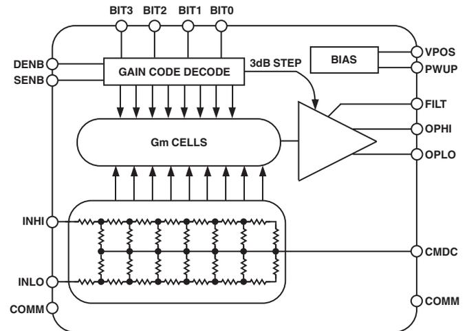
OPHI and OPLO. The overall gain depends upon the source and load impedances due to the resistive nature of the input and output ports.
