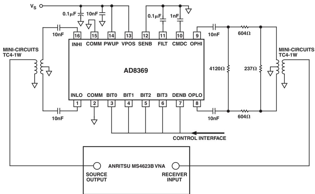
Figure 14. Vector Network Analyzer Setup ( $1\ \text{k}\Omega$ )
