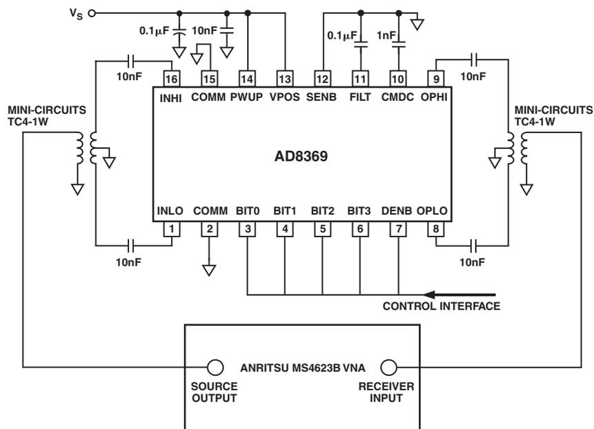
Figure 13. Vector Network Analyzer Setup ( $200\ \Omega$ )
