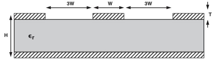
Figure 8. Cross-Sectional View of a PC Board
