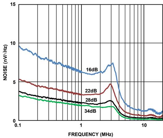
Figure 12. Short Circuit Input-Referred Noise vs. Frequency
