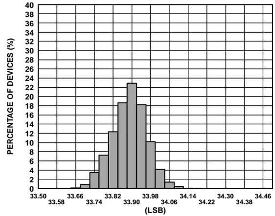
Figure 7. Gain Error Histogram (Gain = 34 dB)
