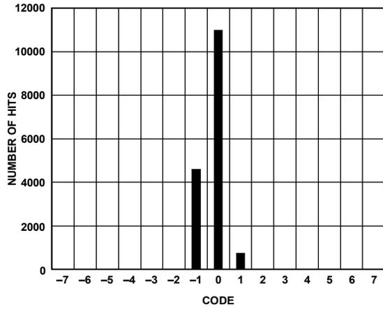
Figure 10. Output Referred Noise Histogram (Gain = 16 dB)
