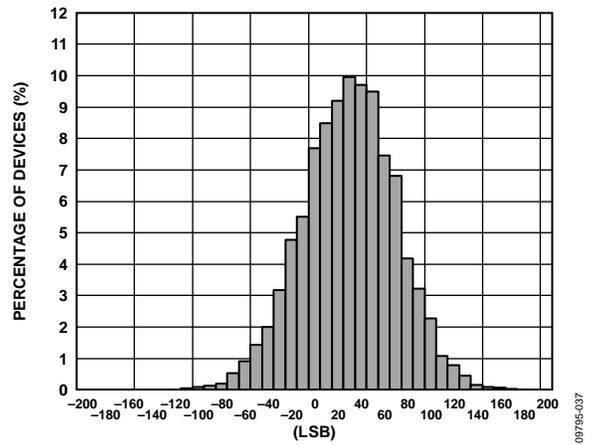
Figure 23. Channel Offset Distribution (Gain = 34 dB)
