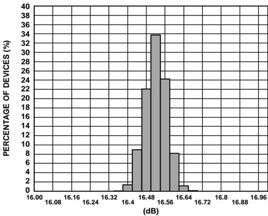
Figure 6. Gain Error Histogram (Gain = 16 dB)
