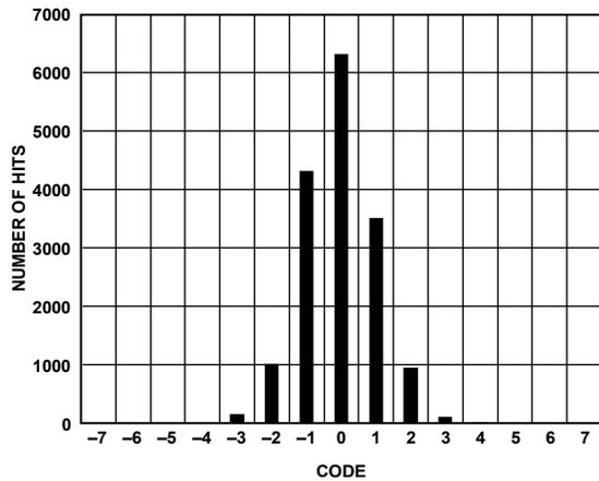
Figure 11. Output Referred Noise Histogram (Gain = 34 dB)
