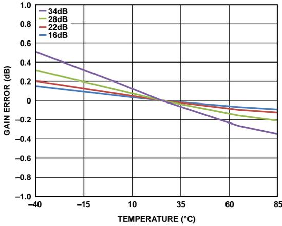
Figure 5. Gain Error vs. Temperature at All Gains
