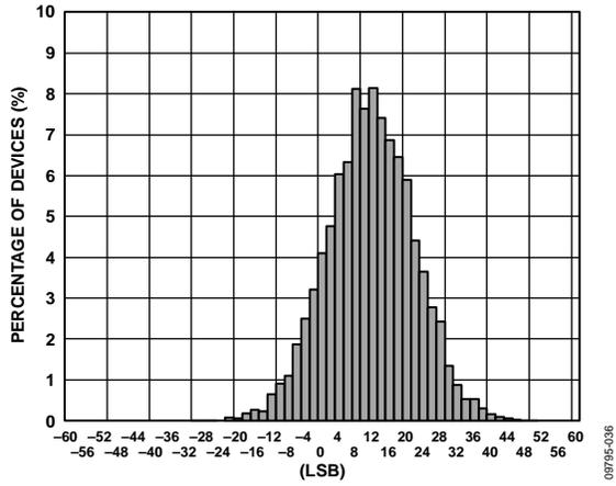
Figure 22. Channel Offset Distribution (Gain = 16 dB)
