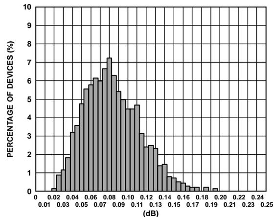
Figure 9. Channel-to-Channel Gain Matching (Gain = 34 dB)
