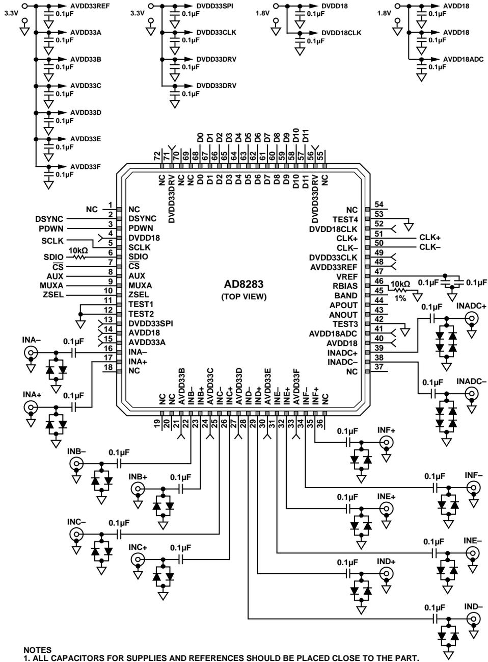
Figure 33. Differential Inputs
