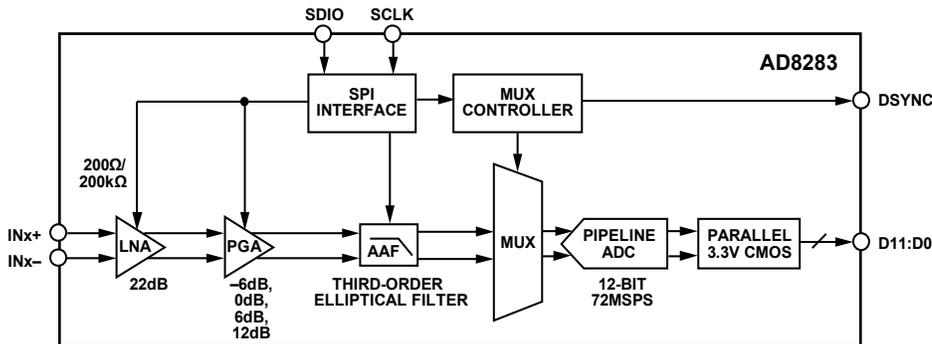
Figure 25. Simplified Block Diagram of a Single Channel
