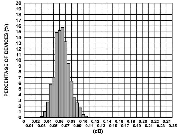
Figure 8. Channel-to-Channel Gain Matching (Gain = 16 dB)
