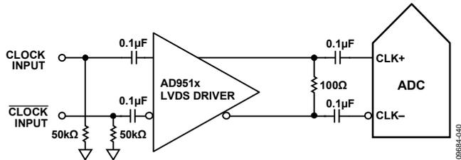
Figure 46. Differential LVDS Sample Clock (Up to 625 MHz)
