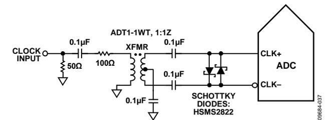
Figure 43. Transformer-Coupled Differential Clock (Up to 200 MHz)
