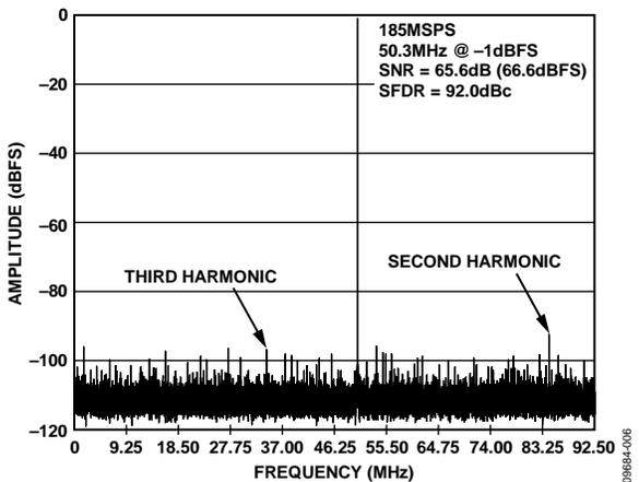
Figure 6. Single Tone FFT,  $f_{IN} = 50.3$  MHz
