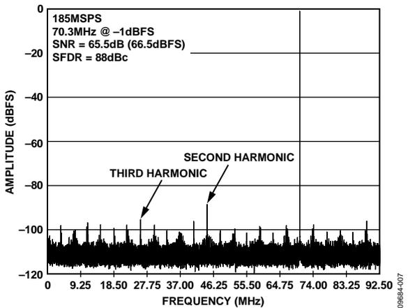
Figure 7. Single Tone FFT,  $f_{IN} = 70.3$  MHz
