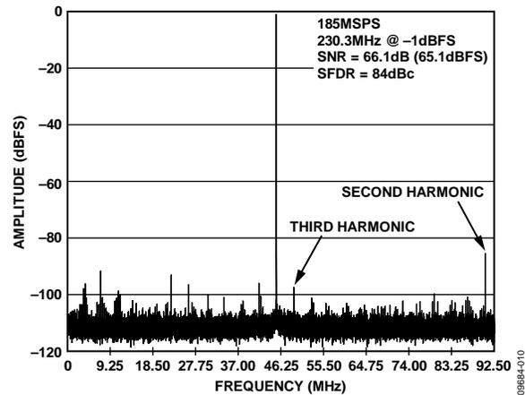
Figure 10. Single Tone FFT,  $f_{IN} = 230.3$  MHz
