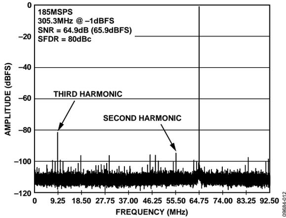
Figure 12. Single Tone FFT,  $f_{IN} = 305.3$  MHz
