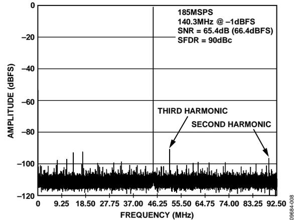
Figure 8. Single Tone FFT,  $f_{IN} = 140.3$  MHz
