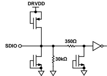
Figure 34. Equivalent SDIO Circuit
