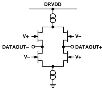
Figure 30. Equivalent LVDS Output Circuit
