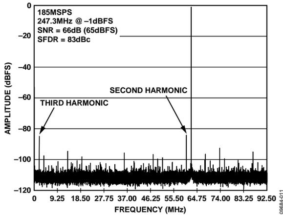
Figure 11. Single Tone FFT,  $f_{IN} = 247.3$  MHz
