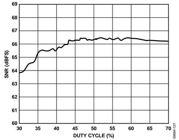
Figure 27. SNR vs. Duty Cycle,  $f_{IN} = 10.3$  MHz
