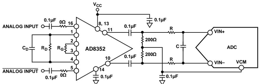
Figure 39. Differential Input Configuration Using the AD8352
