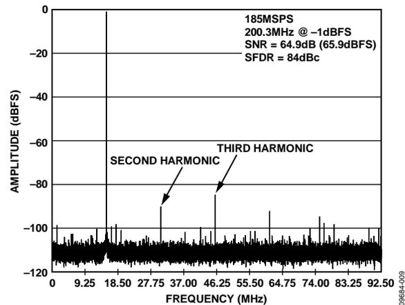
Figure 9. Single Tone FFT,  $f_{IN} = 200.3$  MHz
