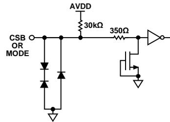
Figure 33. Equivalent CSB and MODE Input Circuit
