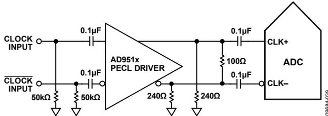
Figure 45. Differential PECL Sample Clock (Up to 625 MHz)
