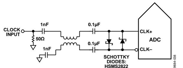
Figure 44. Balun-Coupled Differential Clock (Up to 625 MHz)
