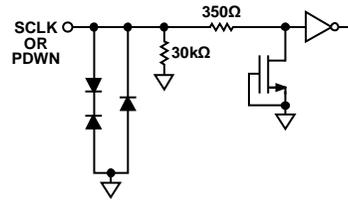
Figure 32. Equivalent SCLK and PDWN Input Circuit
