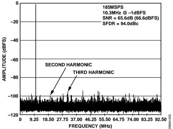
Figure 5. Single Tone FFT,  $f_{IN} = 10.3$  MHz
