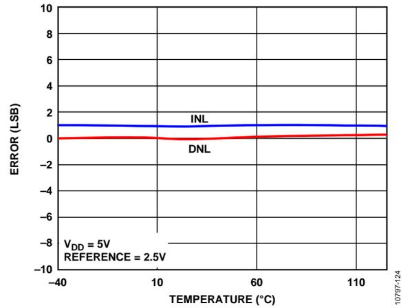
Figure 12. INL Error and DNL Error vs. Temperature
