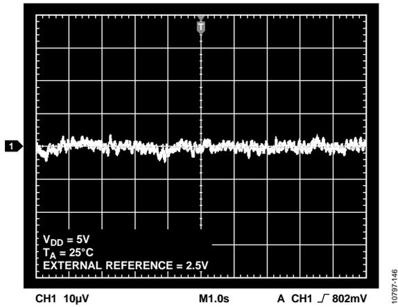
Figure 32. 0.1 Hz to 10 Hz Output Noise Plot
