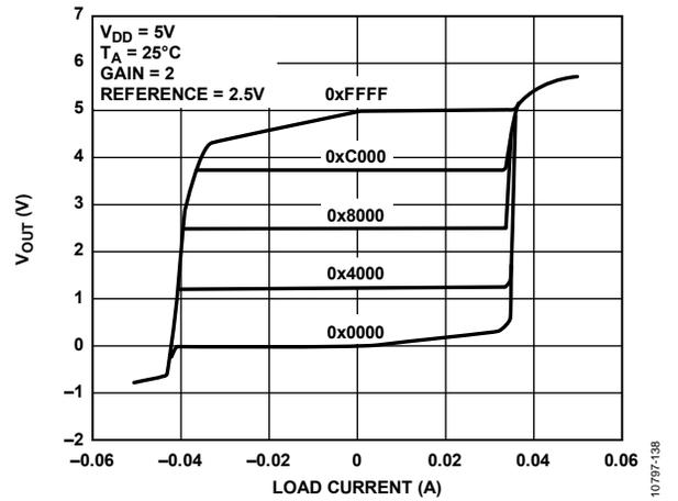
Figure 24. Source and Sink Capability at 5 V
