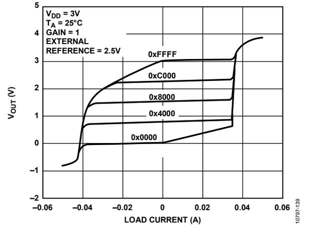
Figure 25. Source and Sink Capability at 3 V
