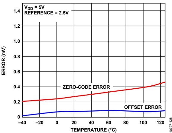
Figure 16. Zero-Code Error and Offset Error vs. Temperature
