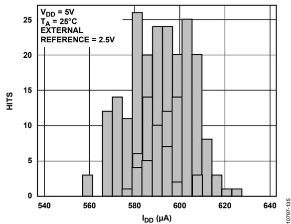
Figure 22.  $I_{DD}$  Histogram
