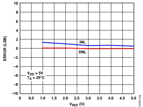
Figure 13. INL Error and DNL Error vs.  $V_{REF}$
