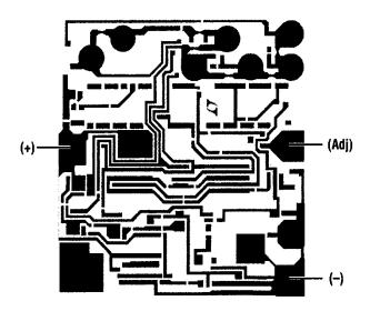
Die bonding pad locations and electrical functions
