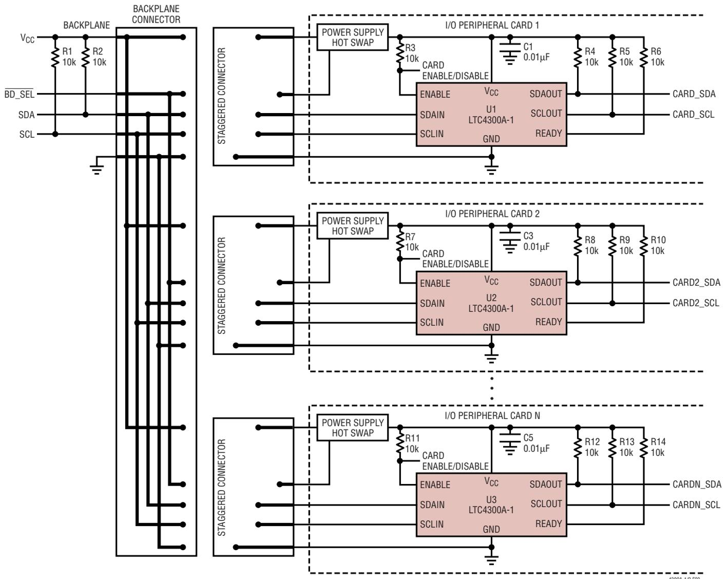
Figure 3. Inserting Multiple I/O Cards into a Live Backplane Using the LTC4300A-1 in a CompactPCI System
