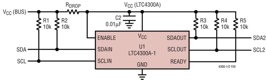
Figure 8. System with Disparate V<sub>CC</sub> Voltages
