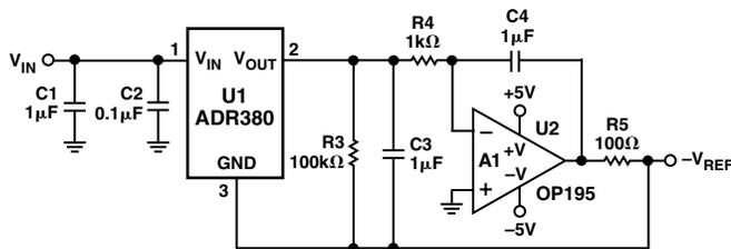
Figure 3. A Negative Precision Voltage Reference Uses No Precision Resistors
