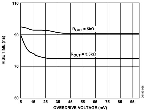
Figure 16. Rise Time vs. Overdrive Voltage (+IN > -IN by Specified V<sub>OD</sub>)
