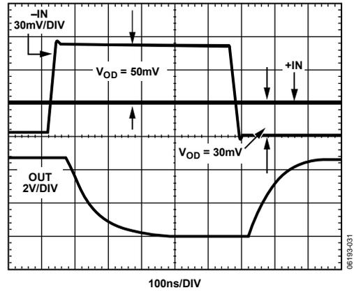
Figure 19. Typical Propagation Delay ( $R_{OUT} = 5\text{ k}\Omega$ )
