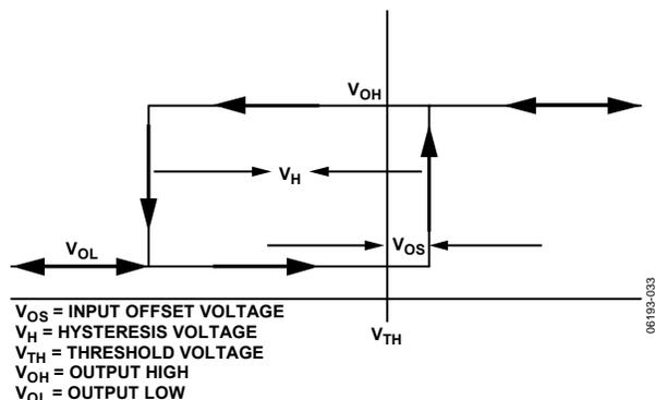
Figure 29. Hysteresis and Input Offset Voltage Definition
