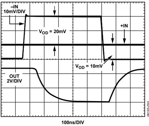
Figure 18. Typical Propagation Delay ( $R_{OUT} = 5\text{ k}\Omega$ )
