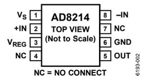
Figure 3. Pin Configuration
