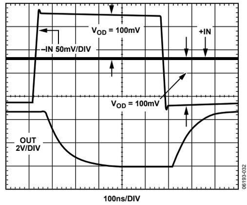
Figure 20. Typical Propagation Delay ( $R_{OUT} = 5\text{ k}\Omega$ )
