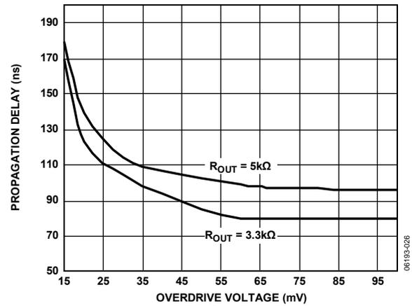
Figure 21. Propagation Delay vs. Overdrive Voltage (-IN > +IN by Specified V<sub>OD</sub>, Output High to Low)
