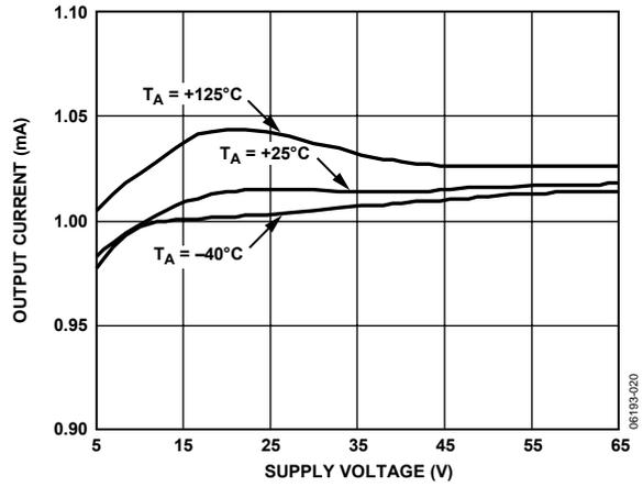
Figure 13. Output Current vs. Supply Voltage (Output High)
