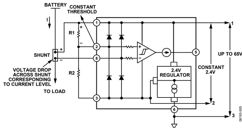
Figure 28. Simplified Schematic
