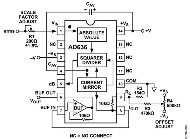
Figure 5. Optional External Gain and Output Offset Trims
