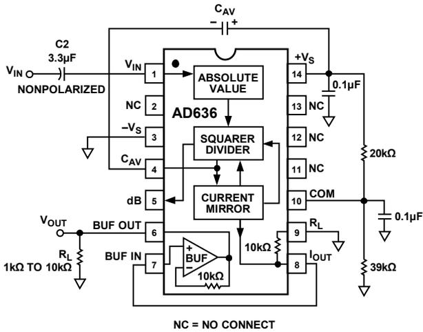
Figure 6. Single-Supply Connection
