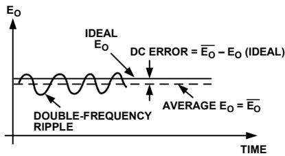
Figure 7. Typical Output Waveform for Sinusoidal Input
