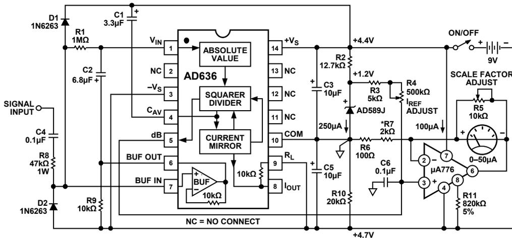
ALL RESISTORS 1/4W 1% METAL FILM UNLESS OTHERWISE STATED EXCEPT \*WHICH IS 2kΩ +3500ppm 1% TC RESISTOR.
