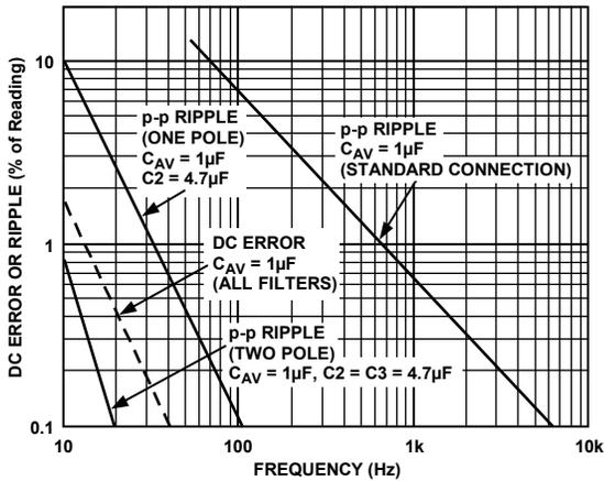
Figure 11. Performance Features of Various Filter Types
