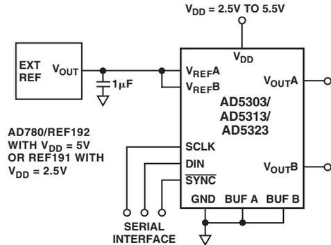
Figure 15. AD5303/AD5313/AD5323 Using External Reference
