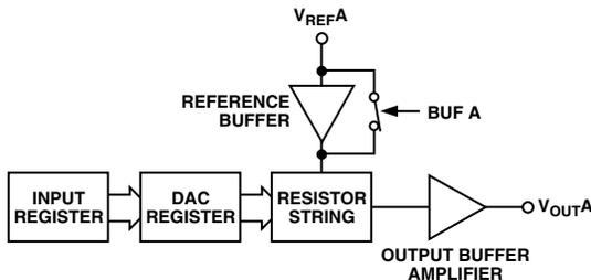
Figure 5. Single DAC Channel Architecture
