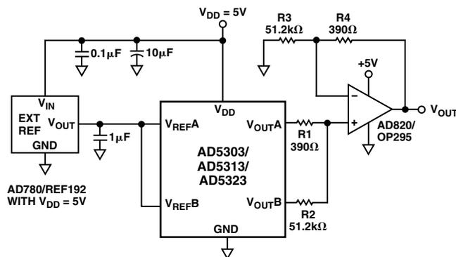
Figure 21. Coarse/Fine Adjustment
