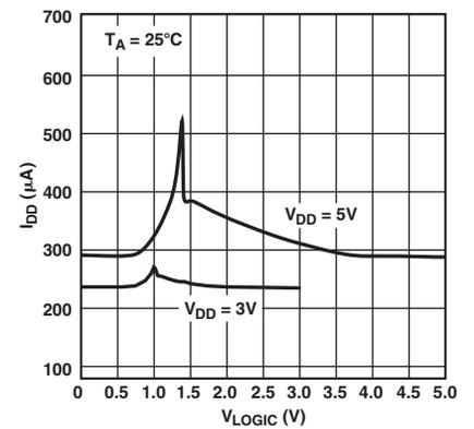
TPC 15. Supply Current vs. Logic Input Voltage
