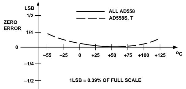
Figure 14. Zero Drift vs. Temperature Performance of AD558
