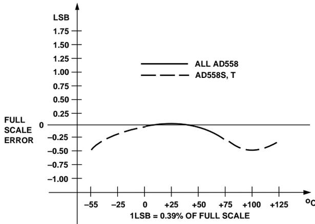
Figure 13. Full-Scale Accuracy vs. Temperature Performance of AD558
