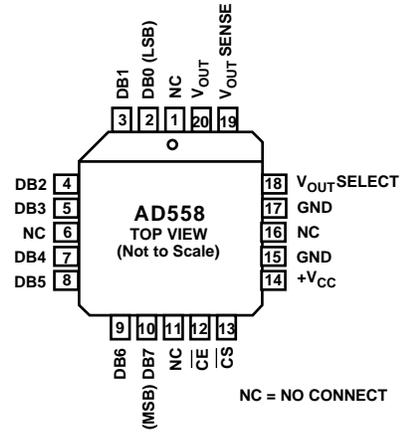
Figure 1b. AD558 Pin Configuration (PLCC and LCC)
