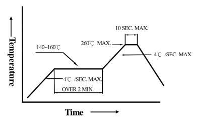
3. DIP soldering (Wave Soldering):
