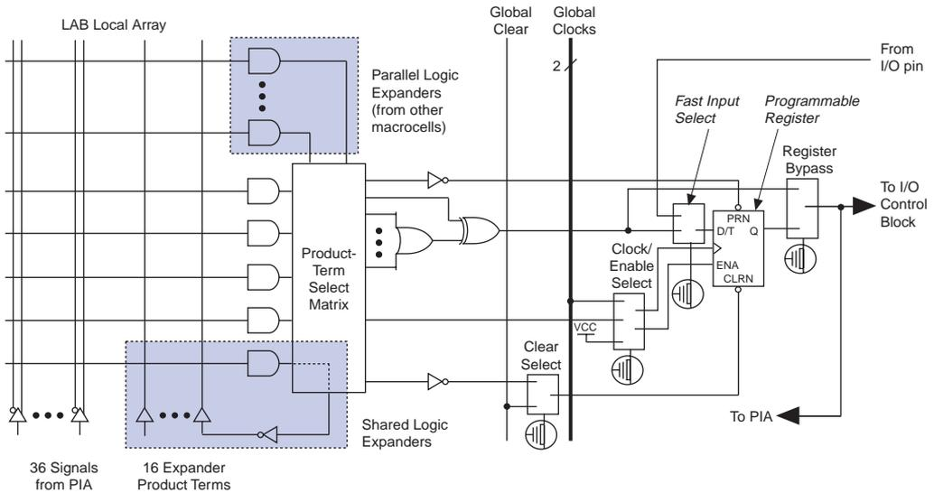
Combinatorial logic is implemented in the logic array, which provides five product terms per macrocell. The product-term select matrix allocates these product terms for use as either primary logic inputs (to the OR and XOR gates) to implement combinatorial functions, or as secondary inputs to the macrocell's register preset, clock, and clock enable control functions.
