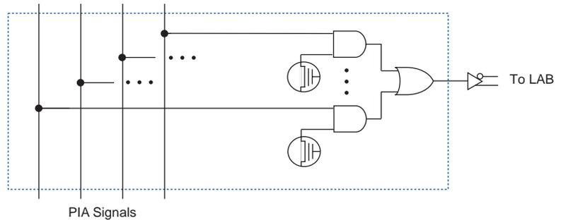
While the routing delays of channel-based routing schemes in masked or FPGAs are cumulative, variable, and path-dependent, the MAX 7000A PIA has a predictable delay. The PIA makes a design's timing performance easy to predict.
