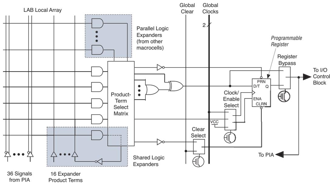
Combinatorial logic is implemented in the logic array, which provides five product terms per macrocell. The product-term select matrix allocates these product terms for use as either primary logic inputs (to the OR and XOR gates) to implement combinatorial functions, or as secondary inputs to the macrocell's register preset, clock, and clock enable control functions.
