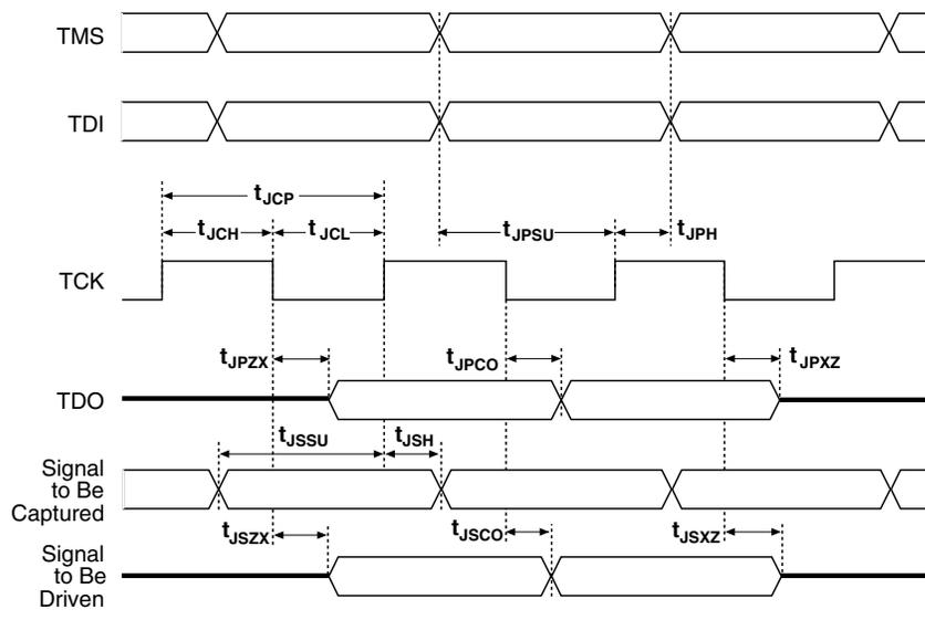
Table 10 shows the JTAG timing parameters and values for MAX 3000A devices.
