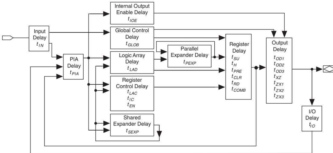
The timing characteristics of any signal path can be derived from the timing model and parameters of a particular device. External timing parameters, which represent pin-to-pin timing delays, can be calculated as the sum of internal parameters. Figure 11 shows the timing relationship between internal and external delay parameters.
