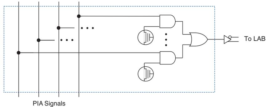
While the routing delays of channel-based routing schemes in masked or FPGAs are cumulative, variable, and path-dependent, the MAX 3000A PIA has a predictable delay. The PIA makes a design's timing performance easy to predict.
