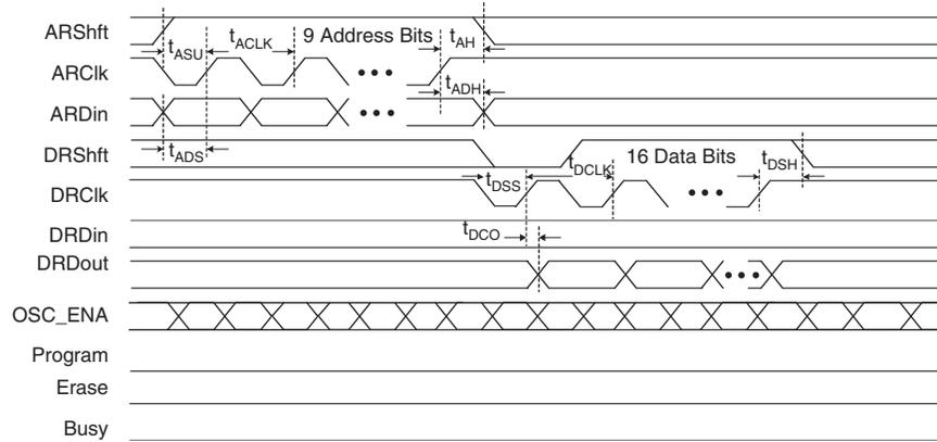
Figure 5-4. UFM Program Waveforms
