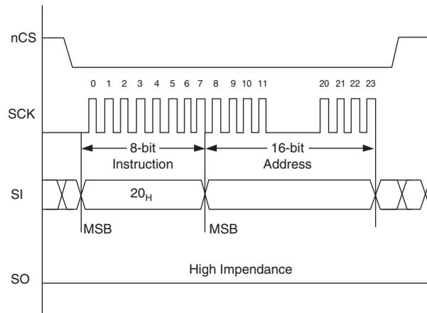
Figure 9-31 shows the SECTOR-ERASE operation sequence for Base mode.
