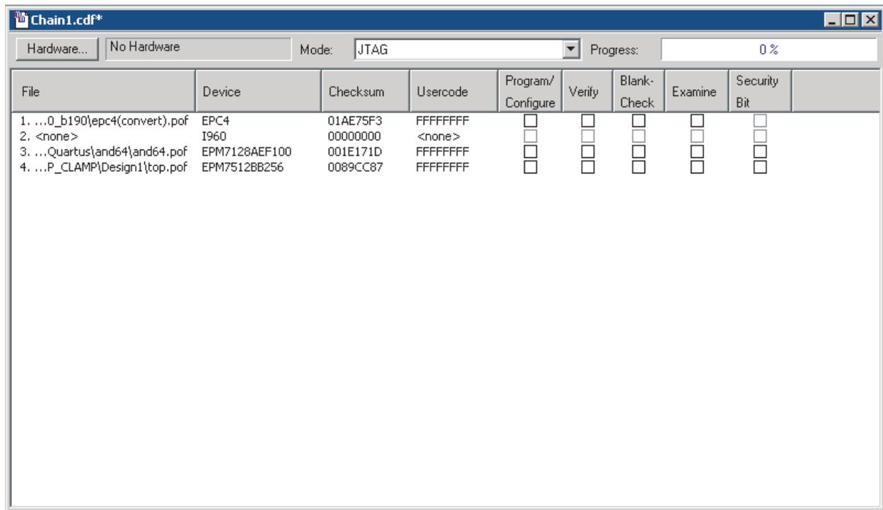
**Figure 14-4.** Generating a JBC File for a Multi-Device JTAG Chain in the Quartus II Software
