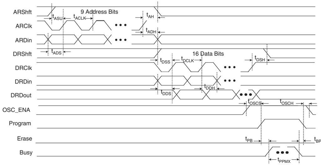
Figure 5-5. UFM Erase Waveform
