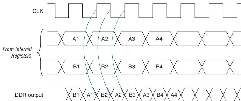
The Stratix II IOE operates in bidirectional DDR mode by combining the DDR input and DDR output configurations. The negative-edge-clocked OE register holds the OE signal inactive until the falling edge of the clock. This is done to meet DDR SDRAM timing requirements.
