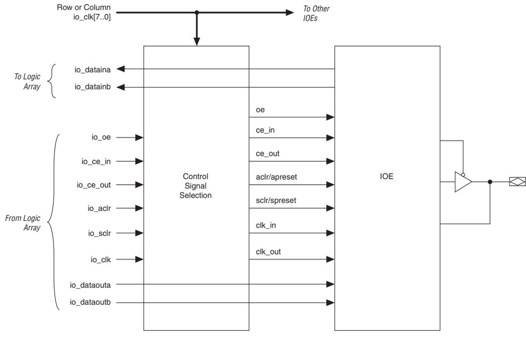
Each IOE contains its own control signal selection for the following control signals: `oe`, `ce_in`, `ce_out`, `aclr/apreset`, `sclr/spreset`, `clk_in`, and `clk_out`. Figure 2–50 illustrates the control signal selection.
