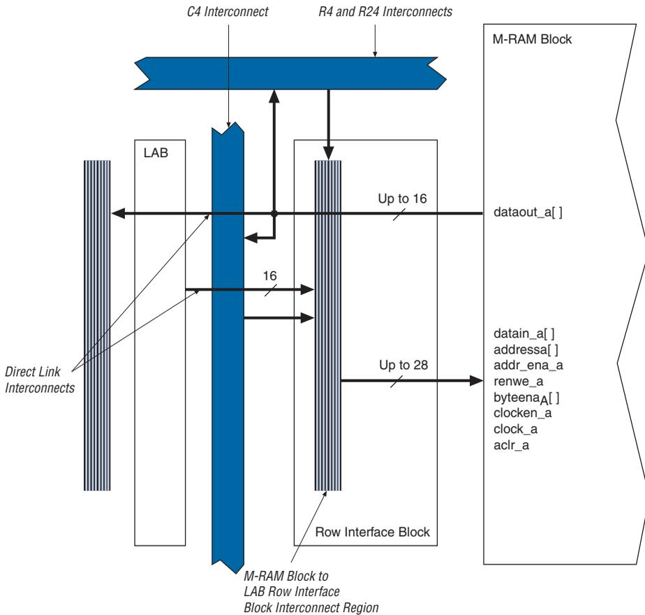
Table 2–4 shows the input and output data signal connections along with the address and control signal input connections to the row unit interfaces (L0 to L5 and R0 to R5).
