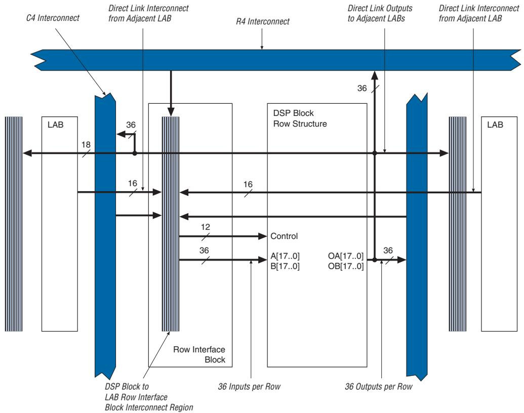
A bus of 44 control signals feeds the entire DSP block. These signals include clocks, asynchronous clears, clock enables, signed/unsigned control signals, addition and subtraction control signals, rounding and saturation control signals, and accumulator synchronous loads. The clock
