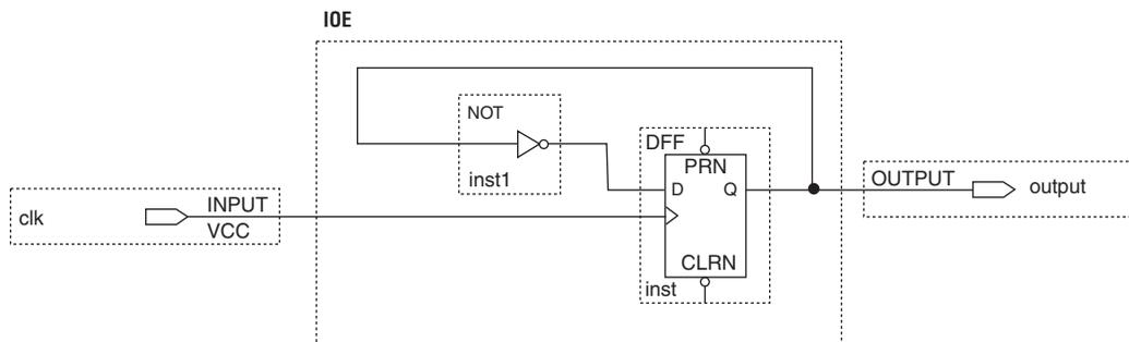
However, when the output is a double data rate input/output (DDIO) signal, both edges of the input clock signal (positive and negative) trigger output transitions (Figure 5–9). Therefore, any distortion on the input clock and the input clock buffer affect the output DCD.
