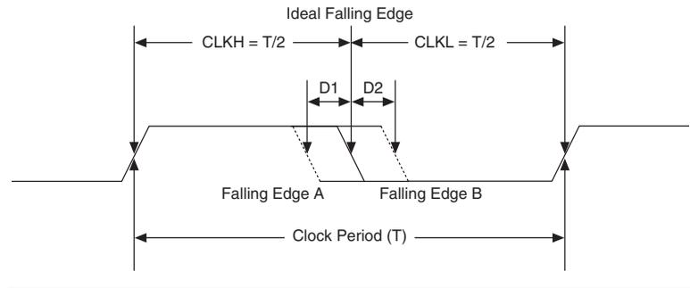
DCD expressed in absolute derivation, for example,  $D1$  or  $D2$  in [Figure 5-7](#), is clock-period independent. DCD can also be expressed as a percentage, and the percentage number is clock-period dependent. DCD as a percentage is defined as
