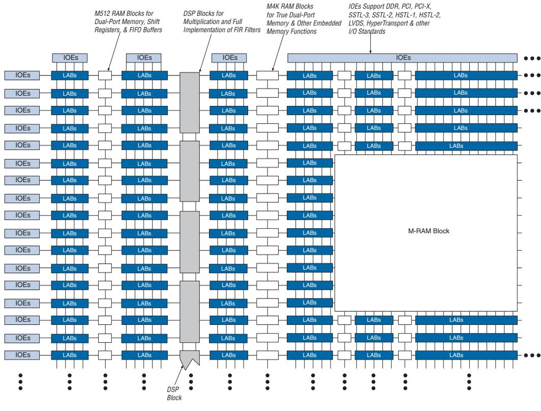
The number of M512 RAM, M4K RAM, and DSP blocks varies by device along with row and column numbers and M-RAM blocks. [Table 2-1](#) lists the resources available in Stratix II devices.
