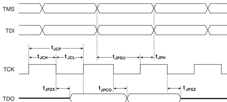
Table 5–102 shows the JTAG timing parameters and values for Stratix II devices.
