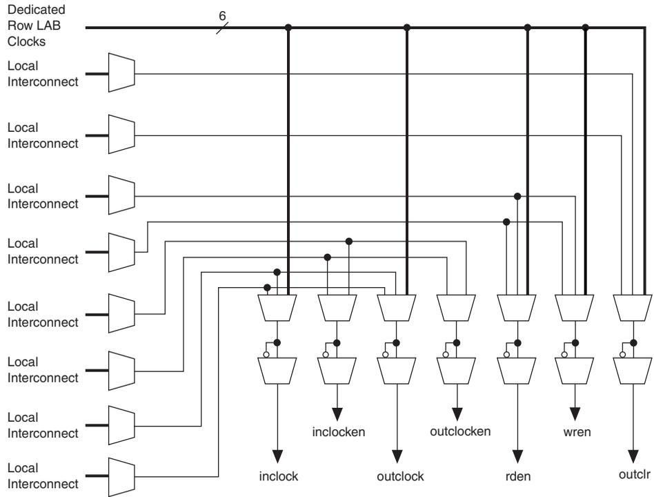
Figure 2–20. M512 RAM Block LAB Row Interface
