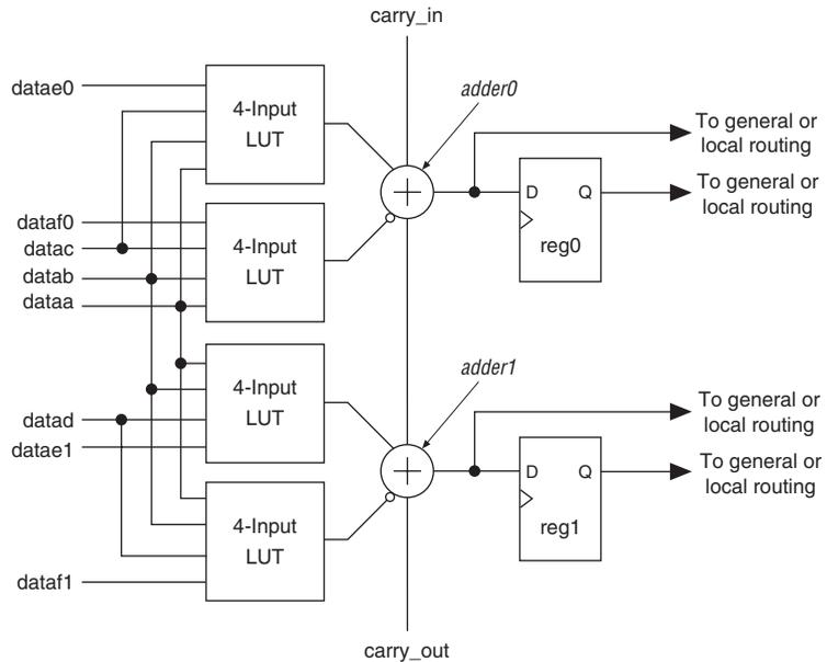
While operating in arithmetic mode, the ALM can support simultaneous use of the adder's carry output along with combinational logic outputs. In this operation, the adder output is ignored. This usage of the adder with the combinational logic output provides resource savings of up to 50% for functions that can use this ability. An example of such functionality is a conditional operation, such as the one shown in Figure 2-12. The equation for this example is:
