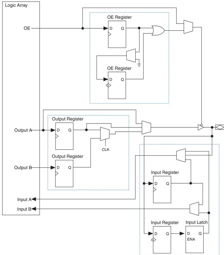
The IOEs are located in I/O blocks around the periphery of the Stratix II device. There are up to four IOEs per row I/O block and four IOEs per column I/O block. The row I/O blocks drive row, column, or direct link interconnects. The column I/O blocks drive column interconnects.
