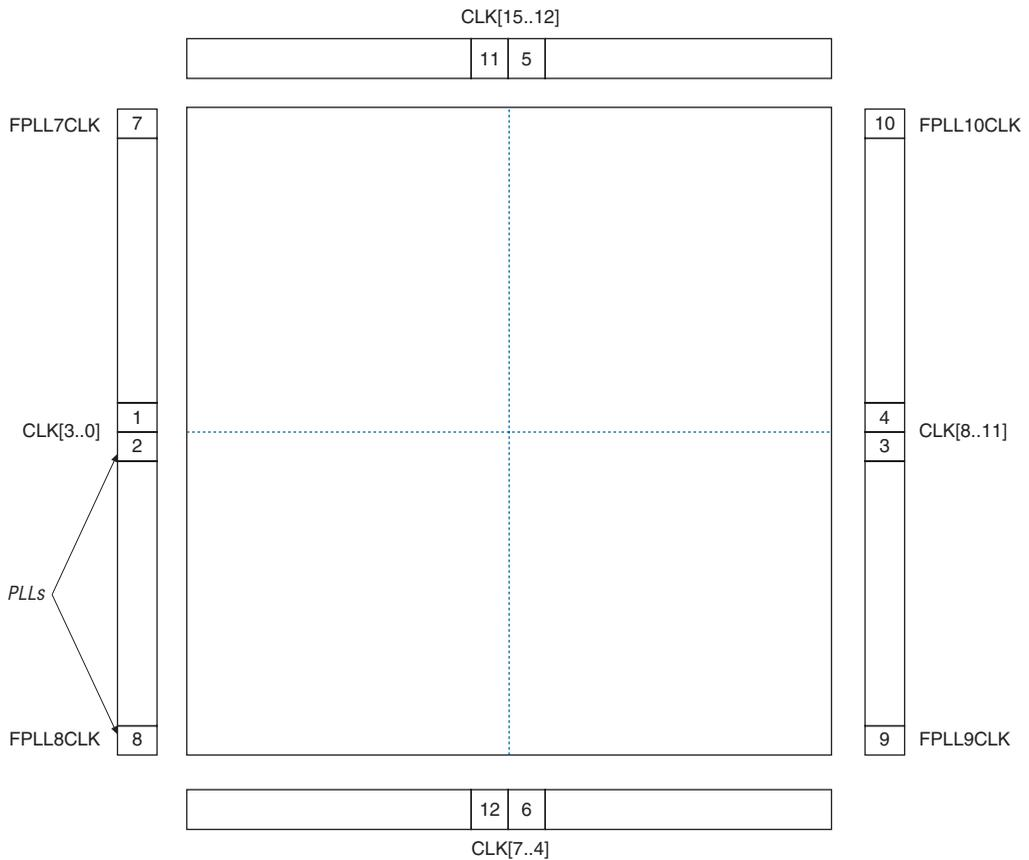
Figures 2–41 and 2–42 shows the global and regional clocking from the fast PLL outputs and the side clock pins. The connections to the global and regional clocks from the fast PLL outputs, internal drivers, and the CLK pins on the left and right sides of the device are shown in table format in Tables 2–11 and 2–12, respectively.
