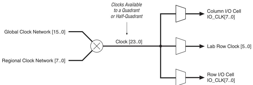
IOE clocks have row and column block regions that are clocked by eight I/O clock signals chosen from the 24 quadrant clock resources. Figures 2-35 and 2-36 show the quadrant relationship to the I/O clock regions.
