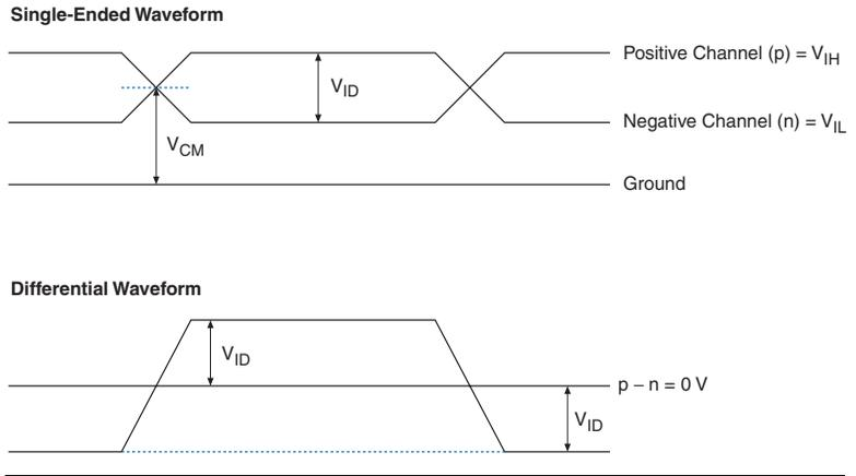
**Figure 5–2. Transmitter Output Waveforms for Differential I/O Standards**
