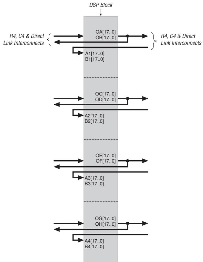
Figure 2–30. DSP Block Interface to Interconnect
