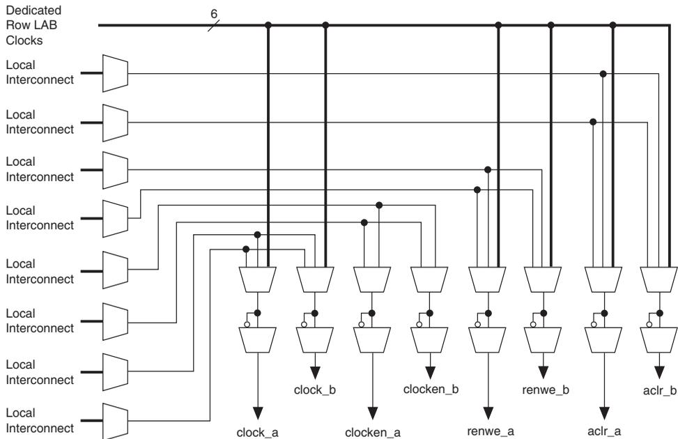
Figure 2–22. M4K RAM Block LAB Row Interface
