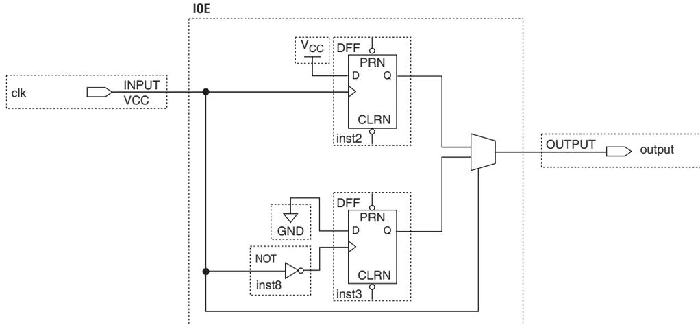
When an FPGA PLL generates the internal clock, the PLL output clocks the IOE block. As the PLL only monitors the positive edge of the reference clock input and internally re-creates the output clock signal, any DCD present on the reference clock is filtered out. Therefore, the DCD for a DDIO output with PLL in the clock path is better than the DCD for a DDIO output without PLL in the clock path.
